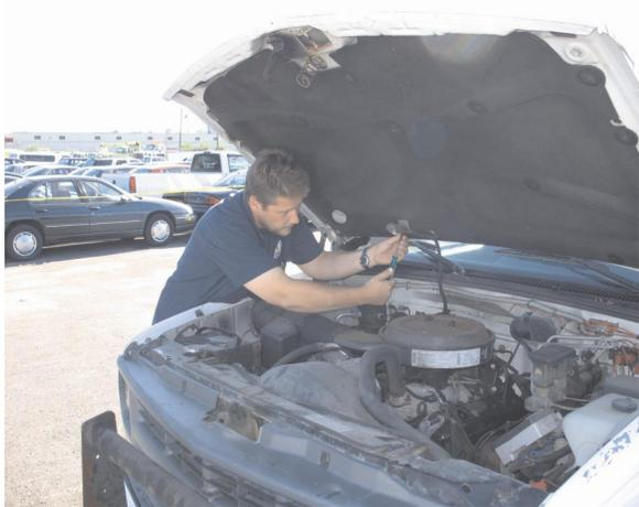
Figure 1. DSS Surplus Vehicle Auction Coordinator Jake Olearchik removes a mercury switch assembly
