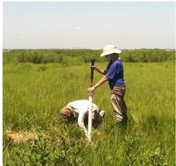
Figure 2 Slide hammer on top of graduated PVC measuring bearing capacity
