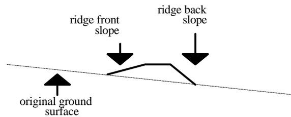
The ridge front slope provides one side of the V-channel while the bottom of the terrace provides the other.
