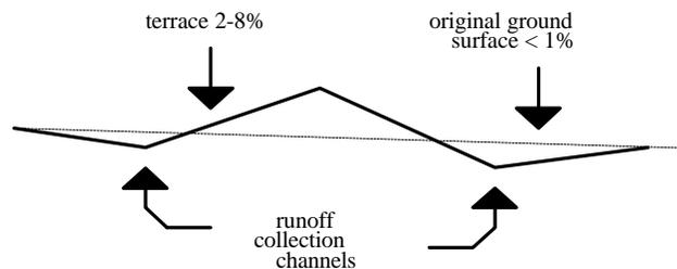
Used where the existing field grade is virtually flat. Construction of individual drainage channels is not necessary because the point where the bottom of adjacent slopes intersect acts as a broad channel.
