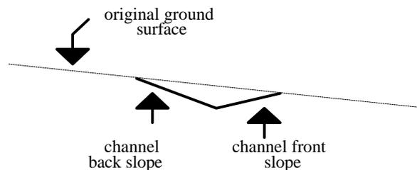
The trough channel is usually constructed by excavating the channel and disposing or stockpiling the soil at another location.
