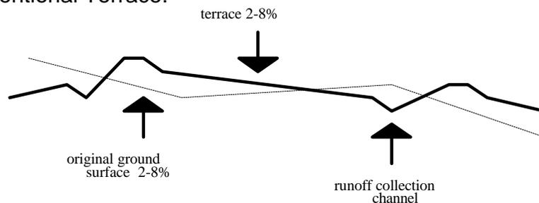
Used when existing field grade generally meets the criteria of 2-8 % slope. Localized cutting and filling is accomplished as necessary to fully meet grade criteria.
