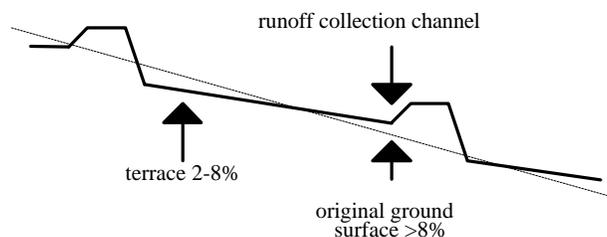
Used where existing field grades are greater than desired (> 8%). Drainage channels are constructed along the lower edge of the higher terrace, adjacent to the step-down to the lower terrace.
