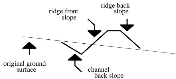
The ridge and trough channel is constructed by excavating the trough and using the excavated soil to form the ridge.
