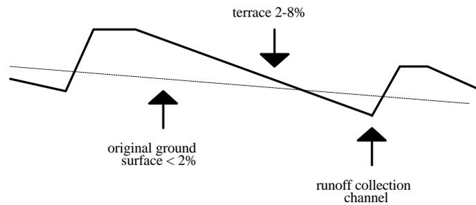
Used where the existing grade is less than desired (< 2%) and it is necessary to increase existing field grades. The front slope of the adjacent terrace provides one side of the runoff collection channel, while the lower portion of the terrace itself provides the other side.
