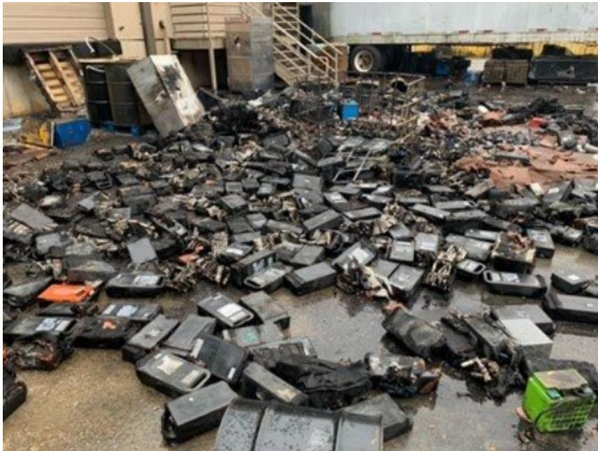
Lithium-ion battery modules and cells lie scattered after they caught fire at a universal waste battery handler in late 2021.
