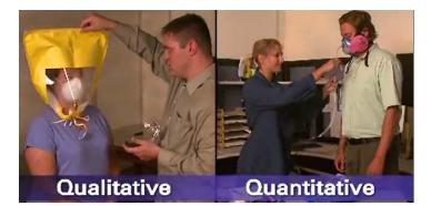
There are two types of fit testing; qualitative and quantitative. Qualitative fit testing is normally used for half-mask respirators, those that just cover your mouth and nose. Half-mask respirators can be filtering facepiece respirators, often called "N95s", as well as elastomeric respirators. Quantitative fit testing can be used for any type of tight-fitting respirator.
