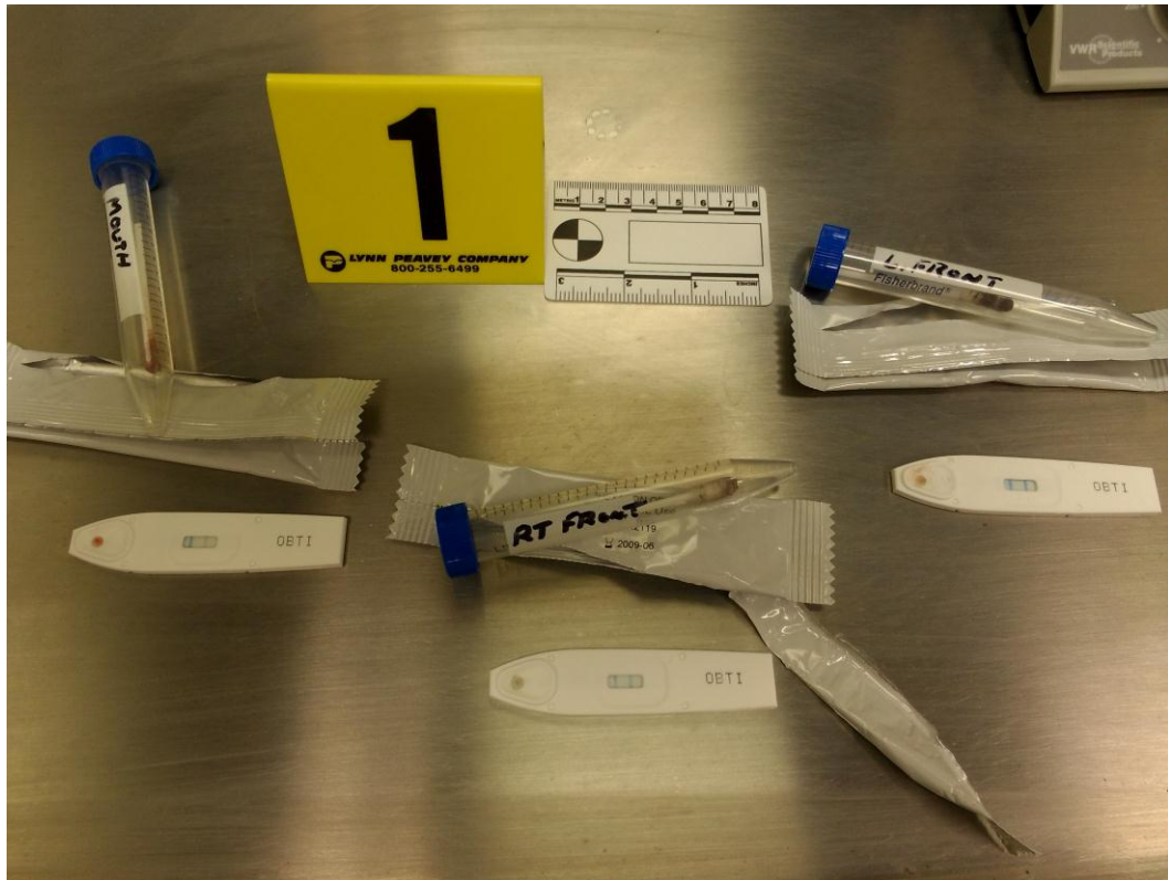
Figure 1: Preliminary test results from three initial swabs taken from the suspected black bears mouth, right paw and left paw. Swabs were tested for the presence of human blood using Hexagon Obti test strips. A positive result is indicated by the presence of two blue lines. All three swabs with their corresponding test strip indicated a positive result for the presence of human blood.
