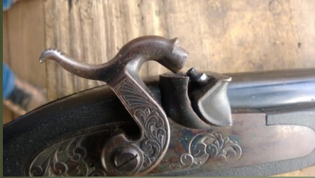
Not Capped and in Safe Position
