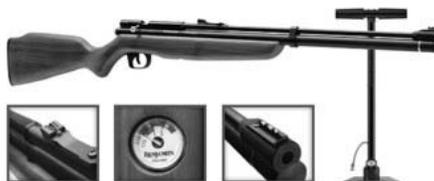
Uses extremely high pressured air (up to 3000 psi) stored in a tank loaded off a scuba tank or specialized hand pump. Every time you squeeze the trigger, a small amount of compressed air is released propelling pellet down barrel.
