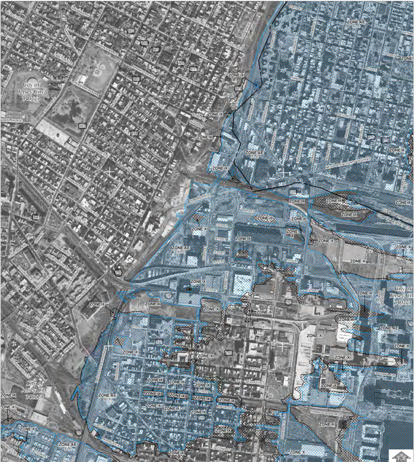
The pale blue dots on this Flood Insurance Rate Map of Hoboken, NJ indicate the Special Flood Hazard Areas (SFHAs). The SFHA (also known as the 1% annual chance flood, 100-year flood, and base flood zone), has historically been subject to a 1% chance of flooding during any given year. In this case, the SFHA is defined as Zone AE, in which the base flood elevations are determined. The areas with the black dots represents areas of historically 0.2% annual chance flood (also known as the 500-year flood zone). Areas without dots have been determined to be outside of the historically 0.2% annual chance floodplain. It is important to highlight that these categories do not include future conditions due to climate change or other factors. (Map obtained through FEMA's Map Service Center, https://msc.fema.gov/portal/home .)
