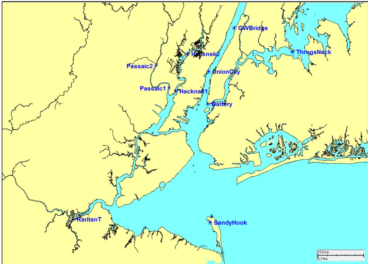
Figure 7. Map of the NOAA tide station locations in the Project area, for comparison of model-predicted and observed tidal elevation harmonic constituents.
