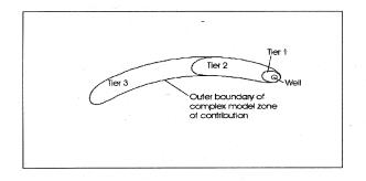
**Figure 5.** Non-CFR model method zone of contribution example.
