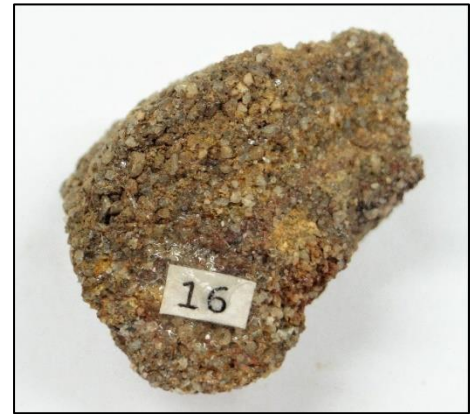
In this ironstone, you can see that it mainly consists of quartz sand with its yellow-white coloration.
