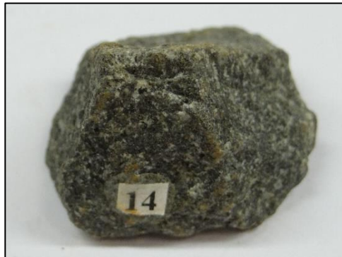
If you look closely at this image of diabase above, you can see the crystals that have formed because of the slow cooling process. The dark specks represent a mineral called pyroxene and the white specks represent the minerals feldspar or plagioclase.
