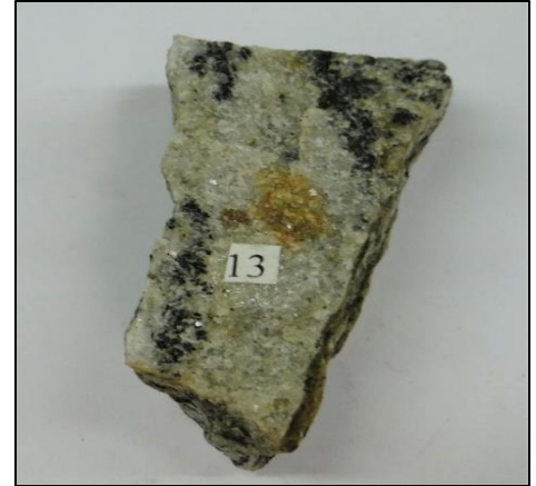
In this gneiss sample, you can see the light-colored crystals, which include quartz and feldspar. You can also see the dark-colored crystals, which include amphibole or biotite mica (iron and magnesium responsible for dark coloration).
