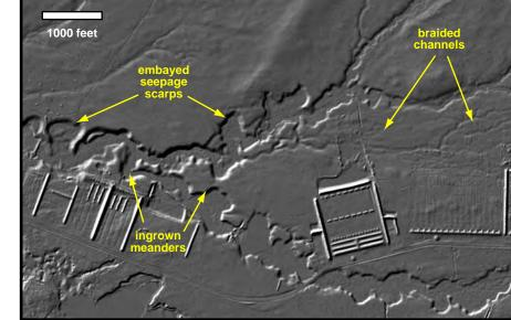
Figure 2. Shaded-relief LiDAR image showing ingrown meanders and embayed seepage scarps at the edge of the modern floodplain, and braided channels on the lower terrace, in the Gaunts Brook valley. Location shown on figure 1.
