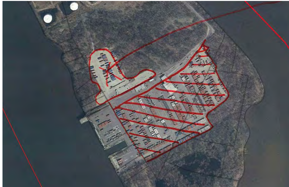
Area shown shaded is area of paving to be removed by Crowley.
