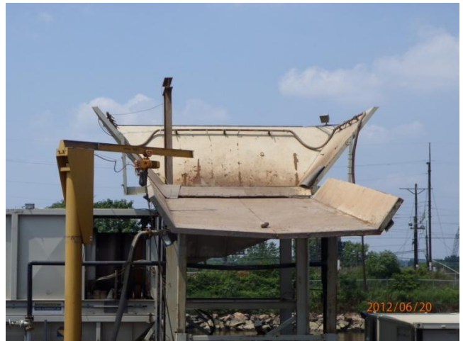
Decontaminated screen hopper
