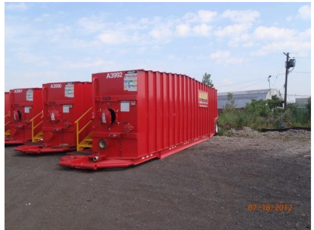
Frac tanks cleaned and awaiting demobilization
