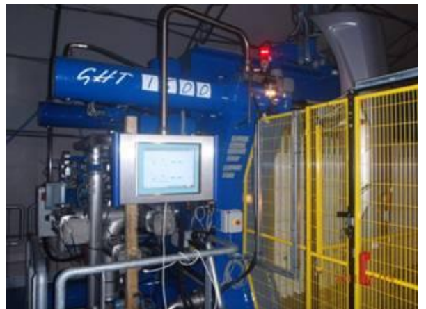
Component testing for a membrane filter press
