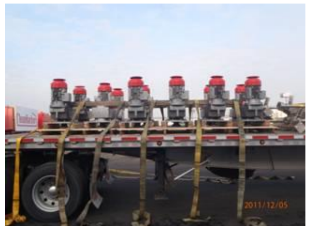
Delivery of agitators for the sludge holding tanks
