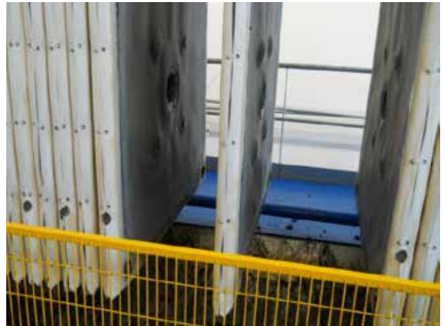
Plates of the membrane filter press
