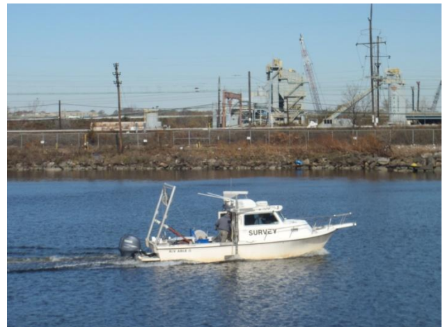
Bathymetry survey of the sediment removal area
