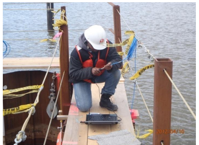
Tide gauge and inclinometer data collection
