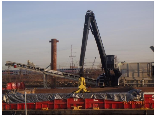
Off-loading sediment for screening and pumping
