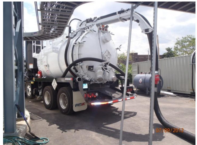
Vacuum truck being used for equipment decontamination
