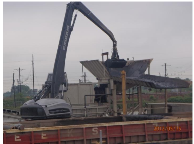
Sediment being loaded into the screening system
