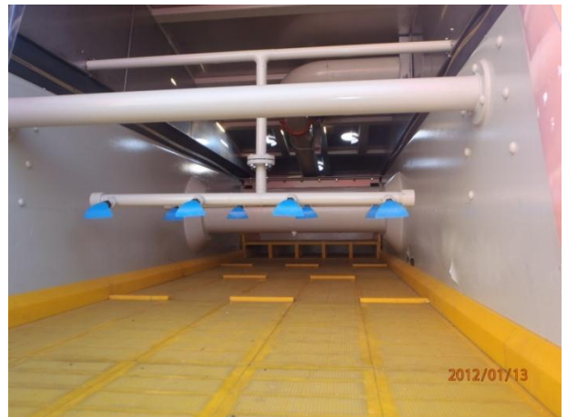
View inside the shaker screen for the sediment processing system
