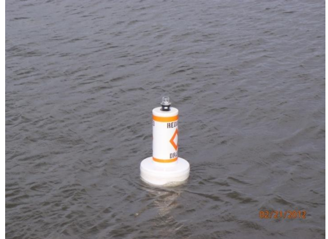
Navigational Buoy with solar light
