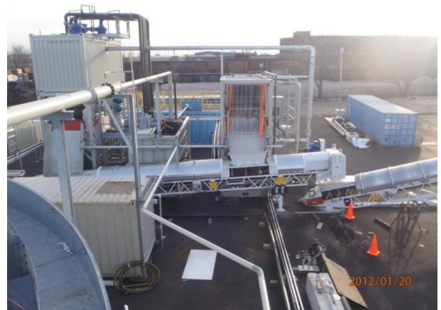
Sand separation system of the sediment processing system
