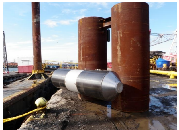
Fish screen for pumps intakes
