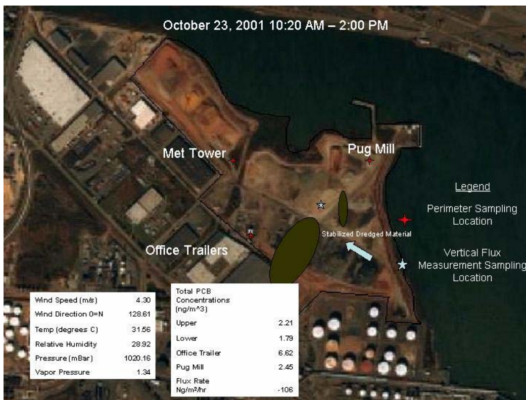
Figure 19. Bayonne landfill site conditions, 23 October 23 2001, 1020 – 1400 hours.
