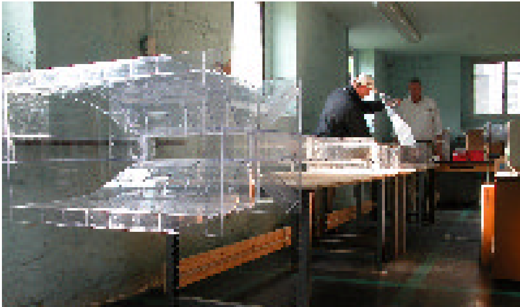
Figure 9. Wind tunnel used to determine sediment-air fluxes of PCBs and Hg from SDM.
