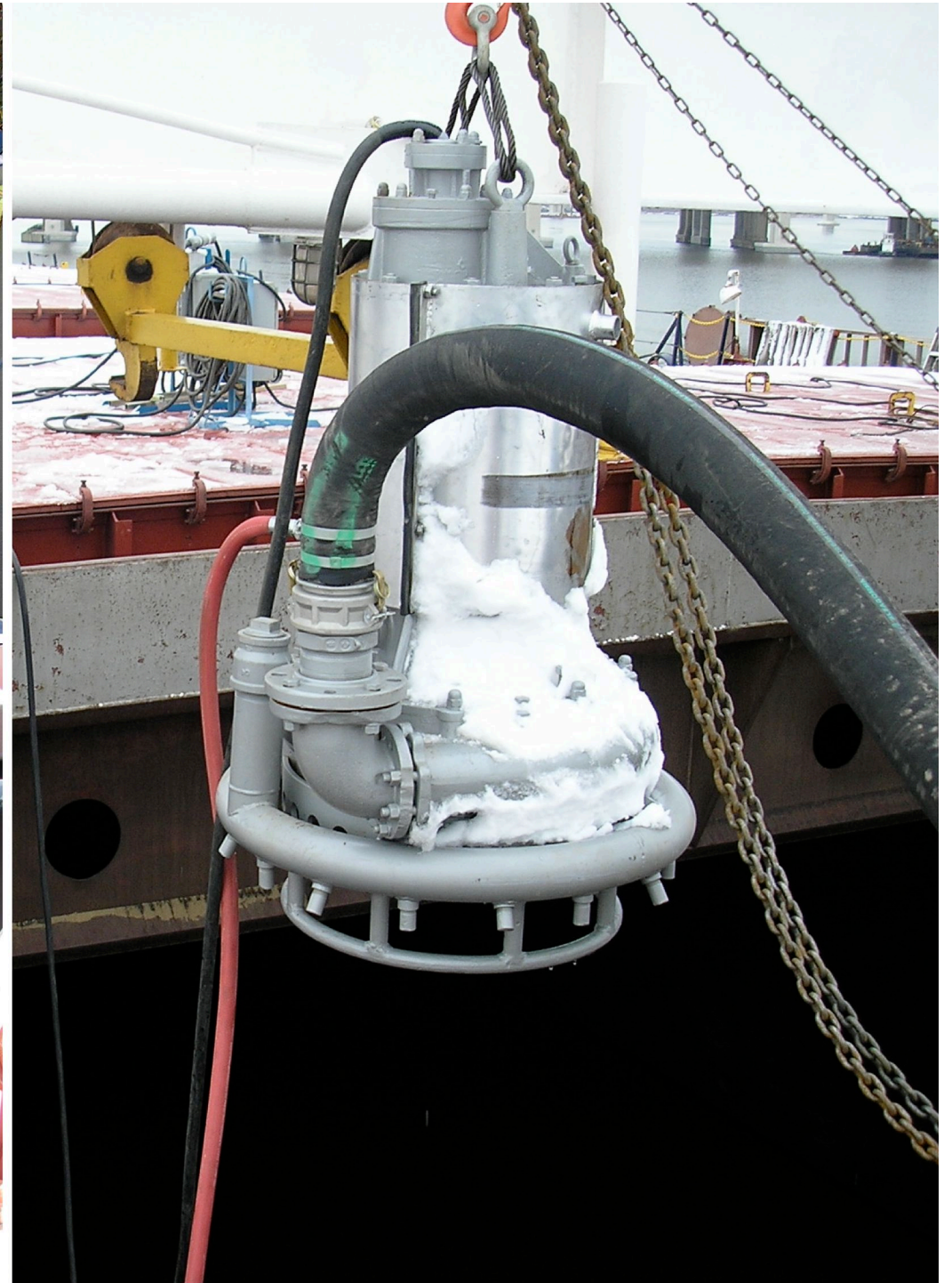
Submersible Pumps for Sediment Mixing and Transfer from Upfront Storage Facility (clockwise from top left: 20 Hp Submersible Pump, Installation of 30 Hp Pump, Recirculation and Mixing of Sediment)
