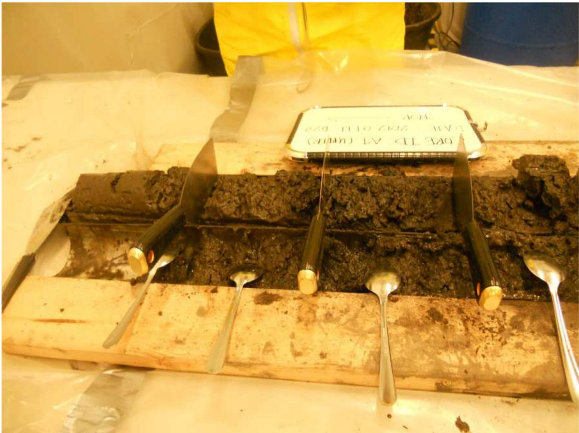
Photograph 38. Sampling tools came into contact with wood boards increasing potential for cross-contamination.
