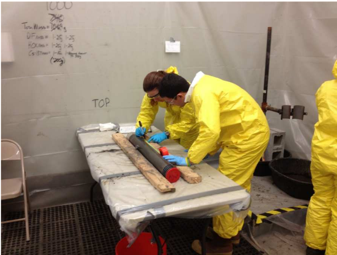
Photograph 33. Cores placed on table and calculated sample segments marked on outside of liner. Plastic sheeting changed occasionally but not prior to every core processed.
