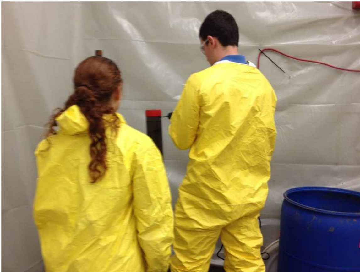
Photograph 30. Drilling through core liner to release excess standing water above sample
