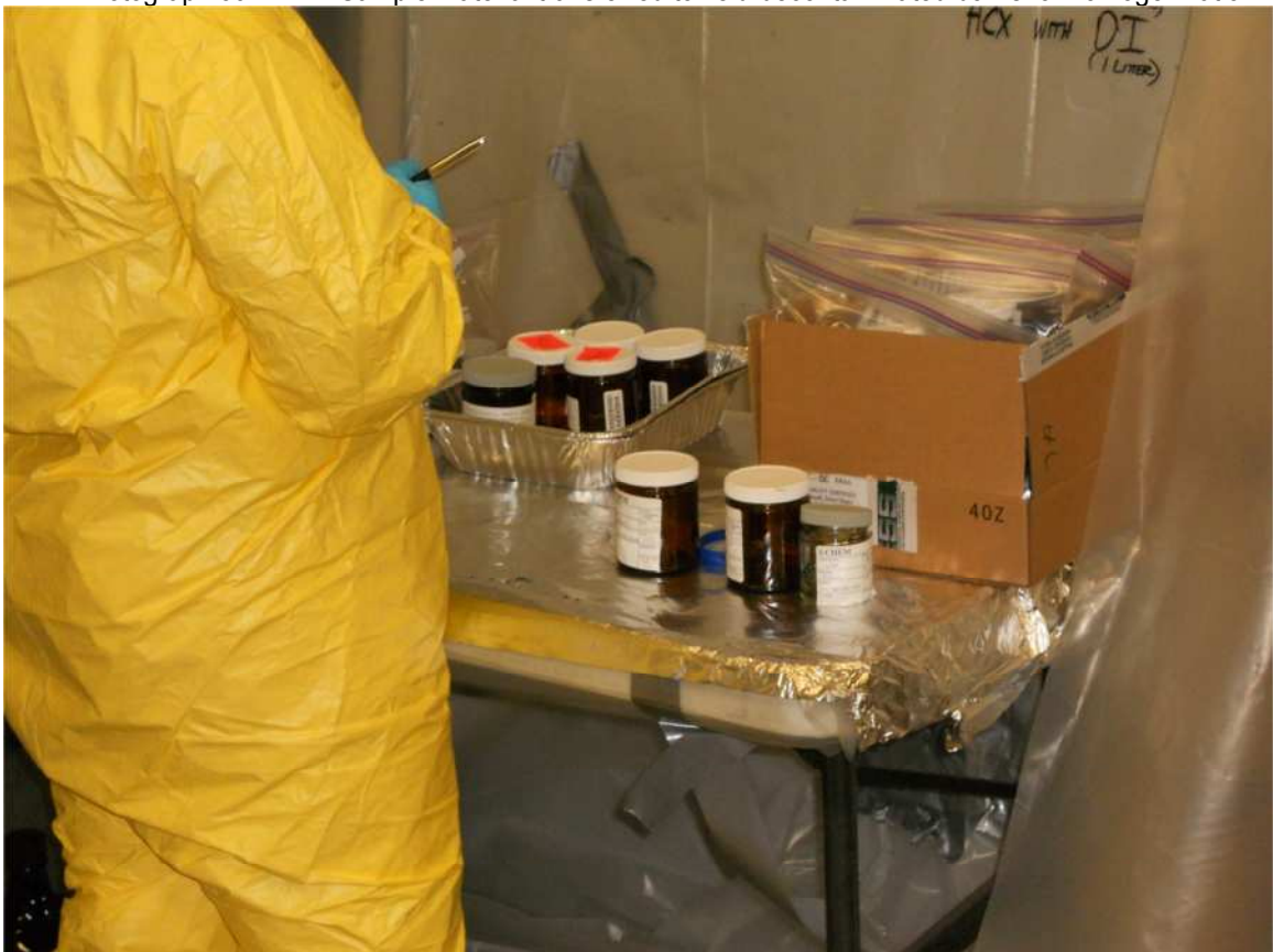
Photograph 40. Hart-Crowser sample bottles filled first (located in aluminum tray). Remaining sample material used to fill Cardno-Entrix and Woodard&Curran sample bottles (three bottles at right).
