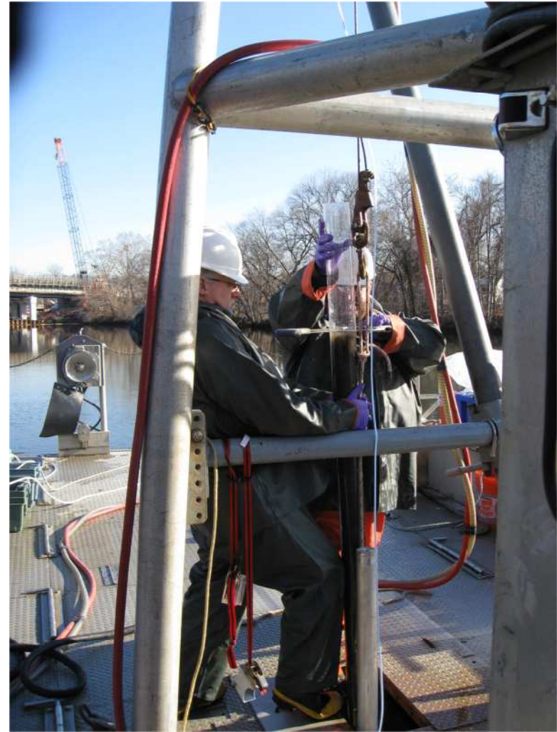
Photograph 12. Cutting recovered core B2 using hacksaw
