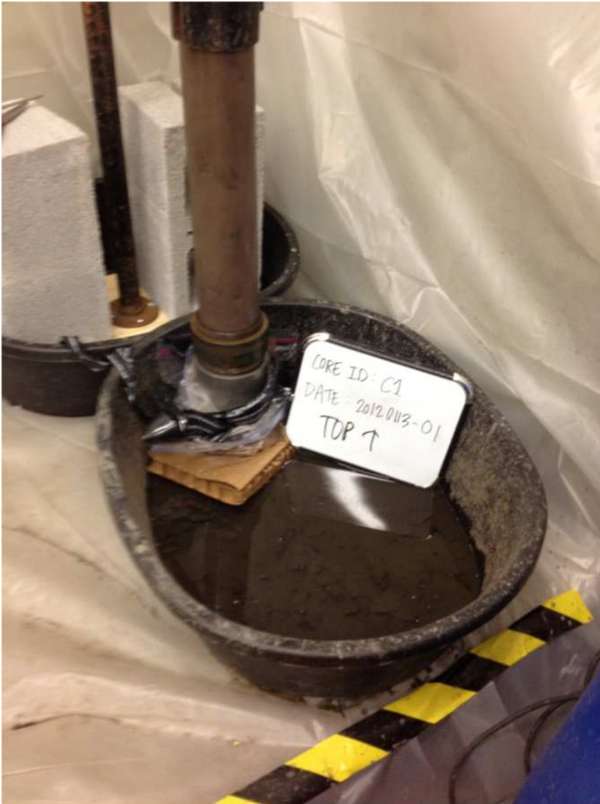
Photograph 41. Sampling crew was unable to remove the cutting head from the core liner recovered at location C1-B.
