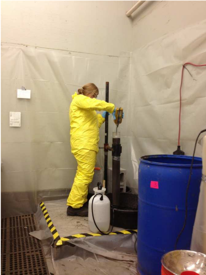
Photograph 31. Core uncapped and organic vapor readings recorded.
