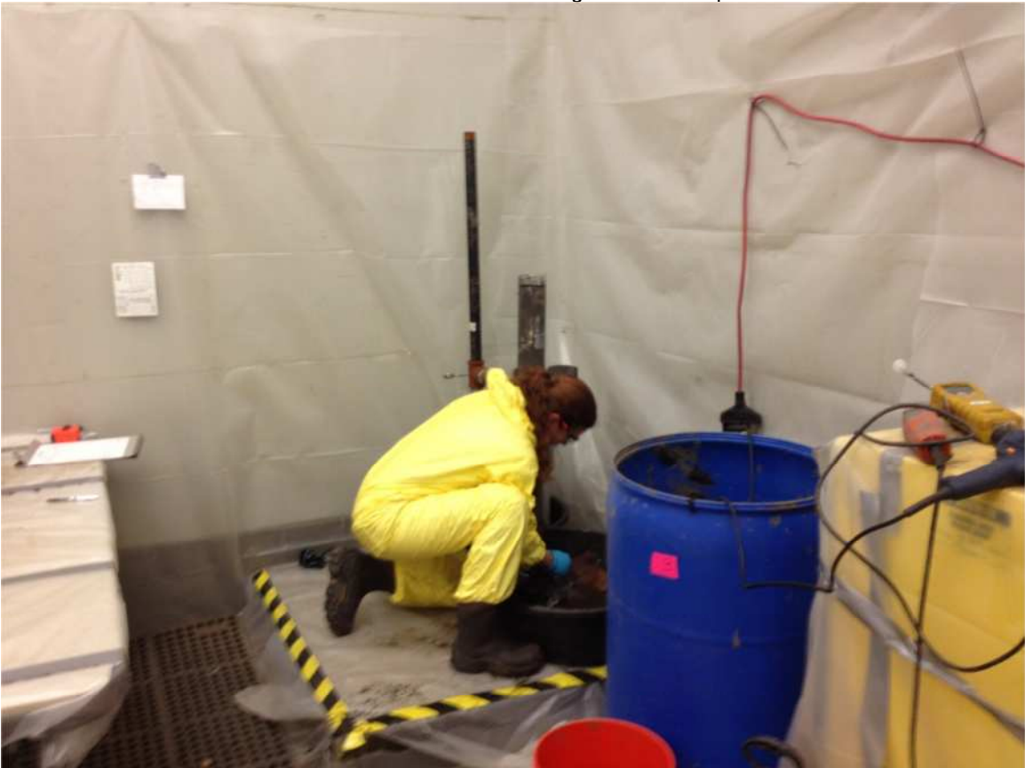
Photograph 48. Core was returned to the support to prevent further spillage. Hart-Crowser estimated 0.5 feet lost.
