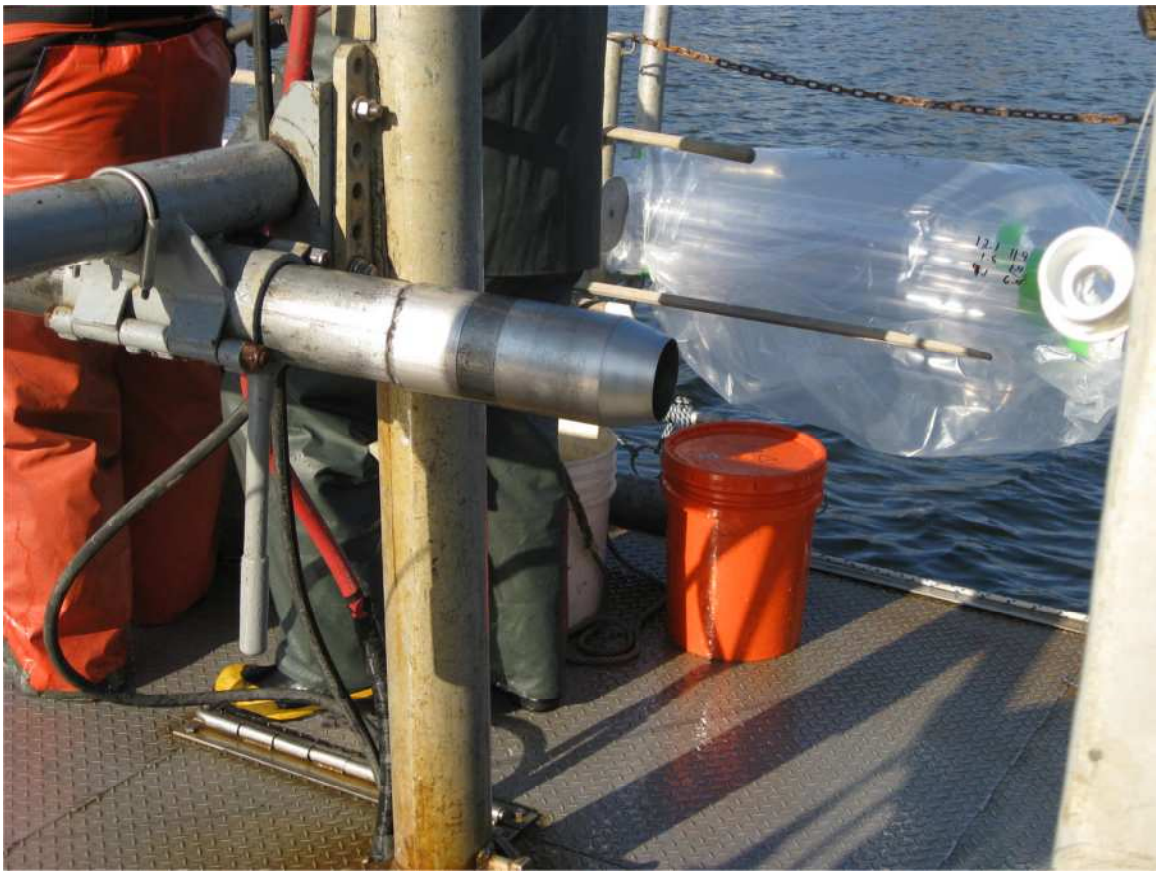
Photograph 3. Cutting shoe/core catcher assembly
