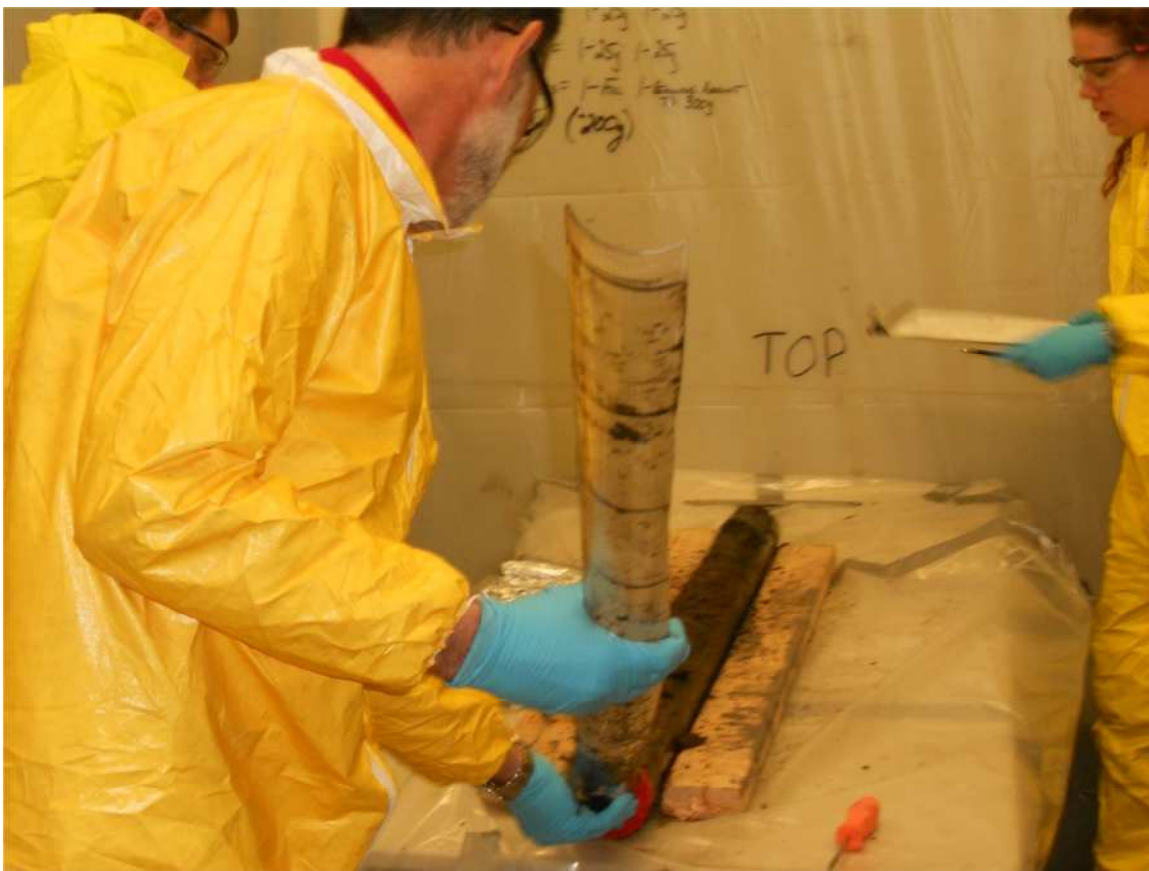
Photograph 35. Exposing core. Sides of core braced with wood boards.
