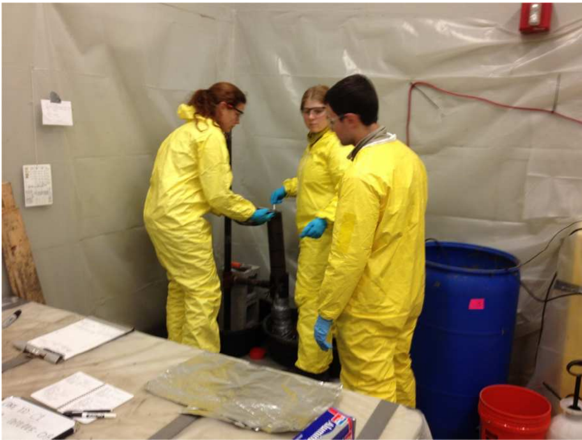
Photograph 49. Core was maintained in vertical position for sampling. Sample material removed from each interval using a ladle.
