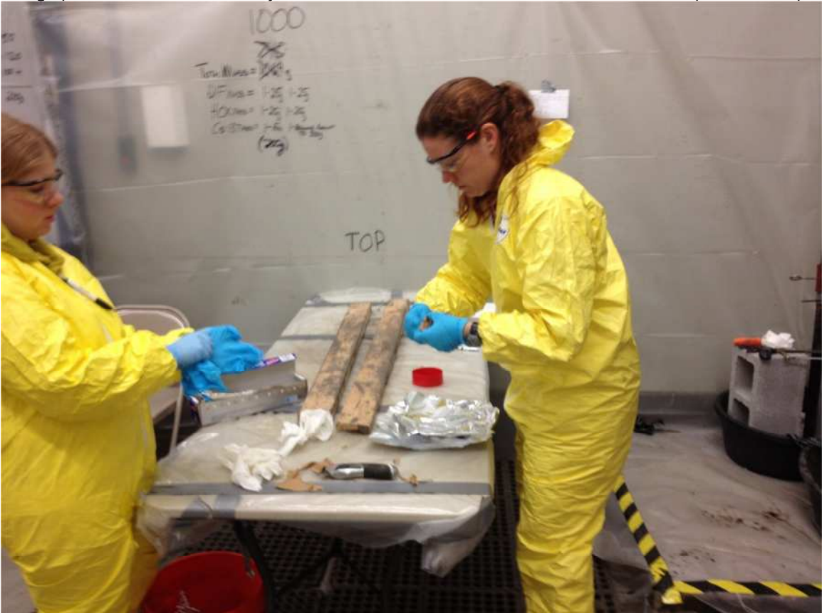
Photograph 44. Samplers fabricated a temporary plug of aluminum foil and cardboard to keep material stable while transferring the core to the processing table.
