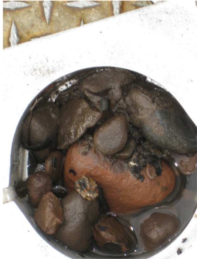
Photograph 16. Gravel and cobbles trapped in core catcher at location C2
