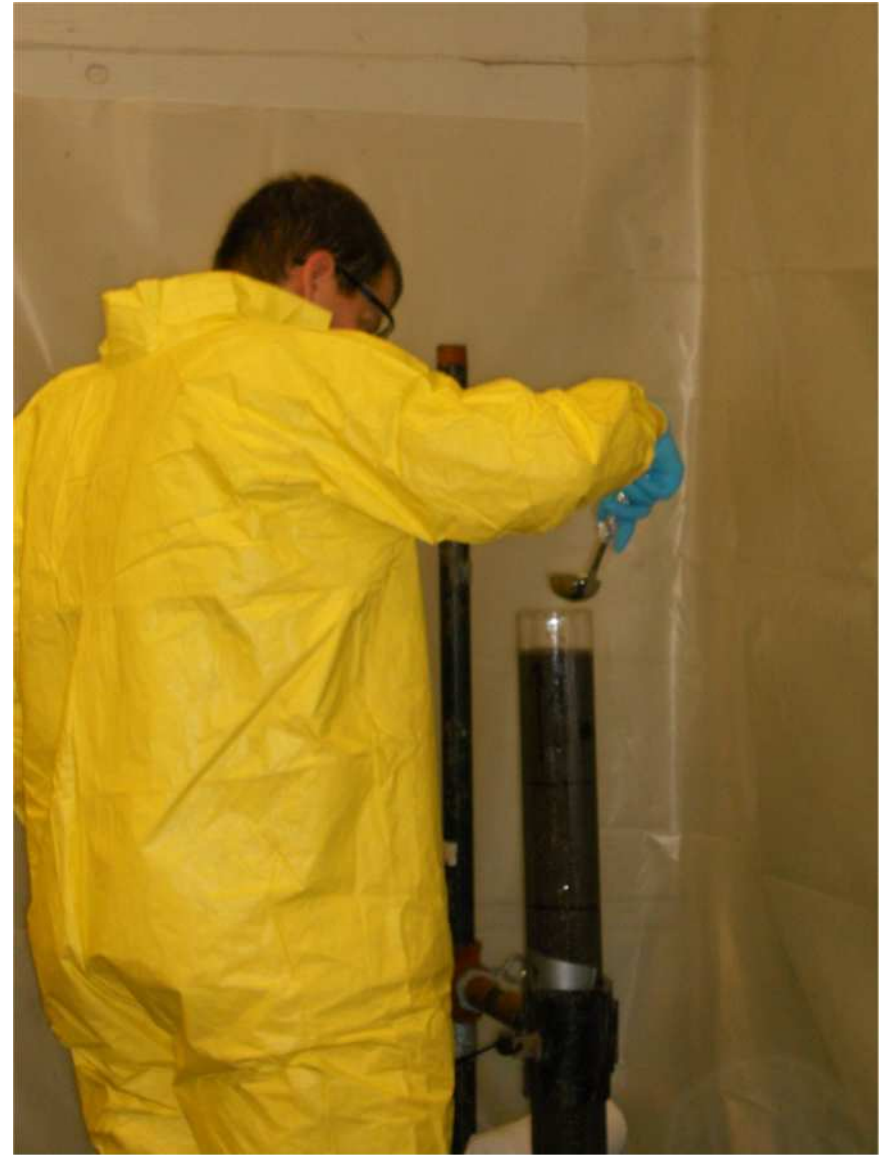
Photograph 32. Excess liquid and flakes of cut core liner removed from top of sample using a stainless-steel ladle.
