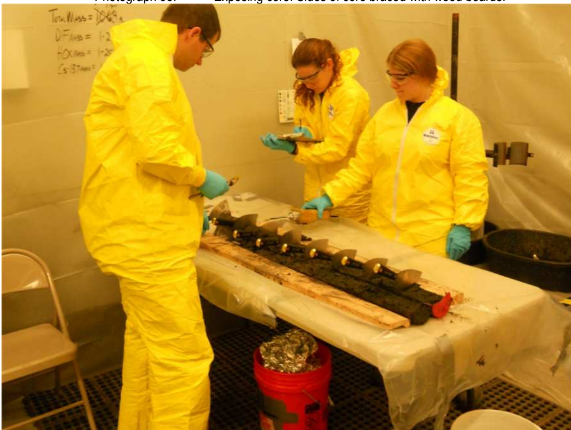
Photograph 36. Spatulas placed to demarcate each sample segment. Organic vapor readings taken above each segment. Same wood boards reused to brace each core.
