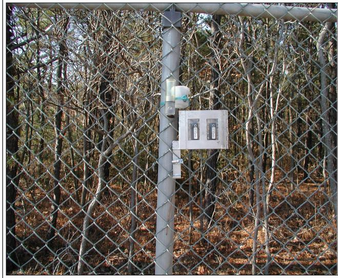
**Figure 3– TLD Used in the Environment**
