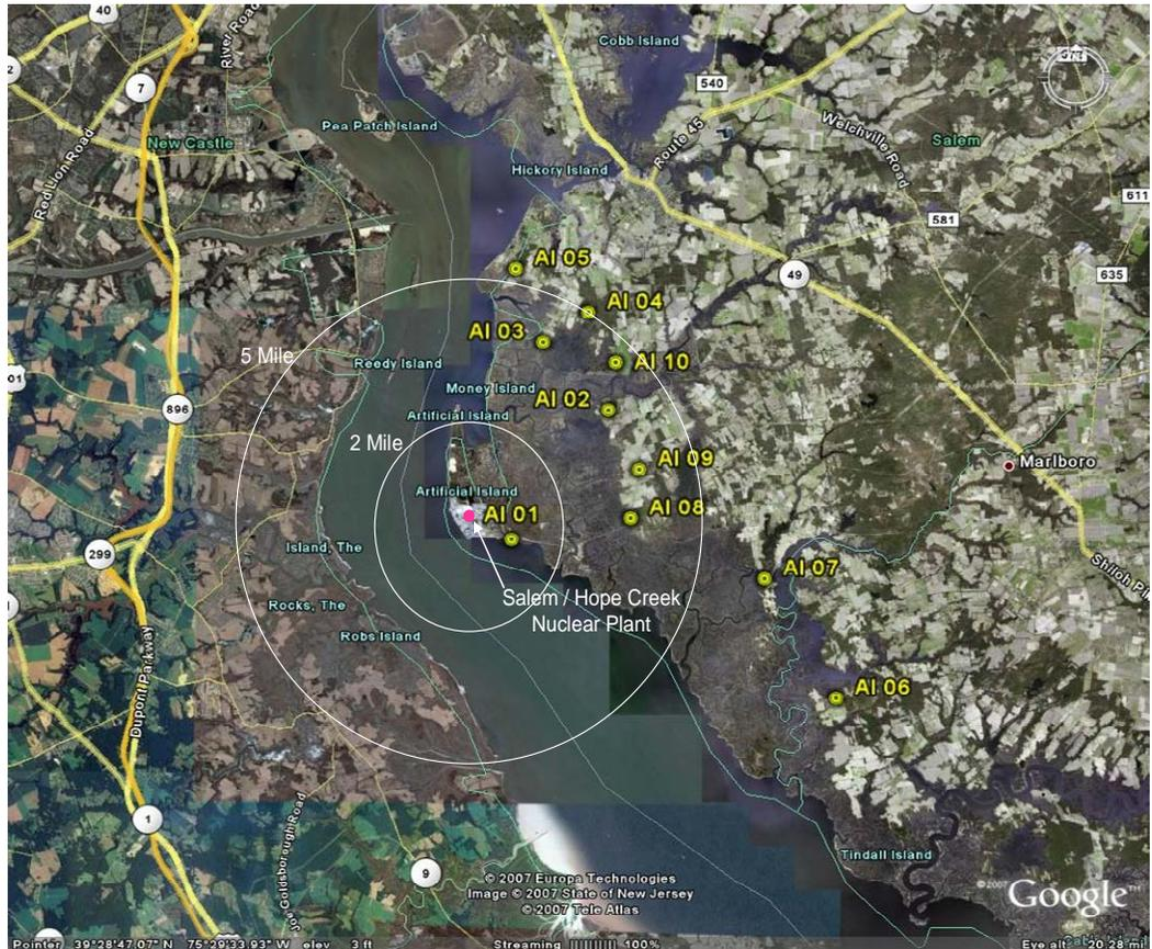
Figure 10 – CREST and Thermoluminescent Dosimeter Locations, Salem/Hope Creek
