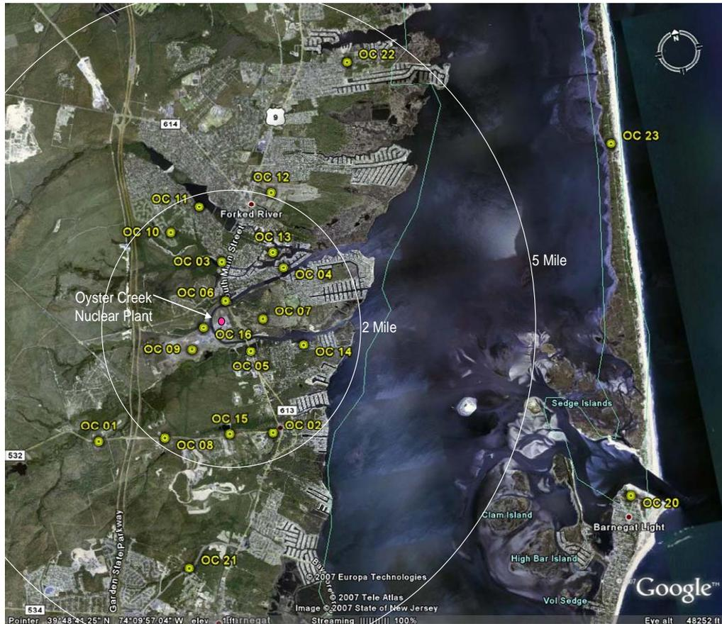
**Figure 7 – CREST and Thermoluminescent Dosimeter Locations
