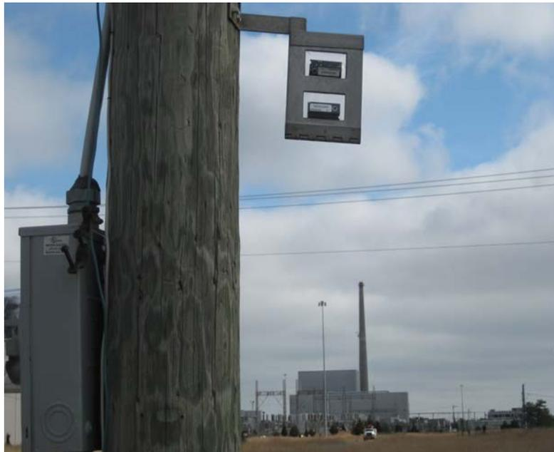
**Figure 3 – TLD Used in the Environment**
