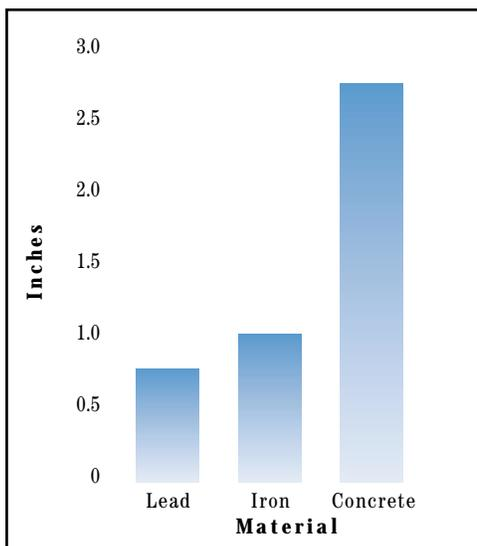
**Figure 1. Shielding Materials and Their Half-Thicknesses for Gamma Radiation**
