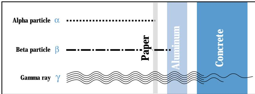
**Figure 2. Types of Radiation and Shielding**
