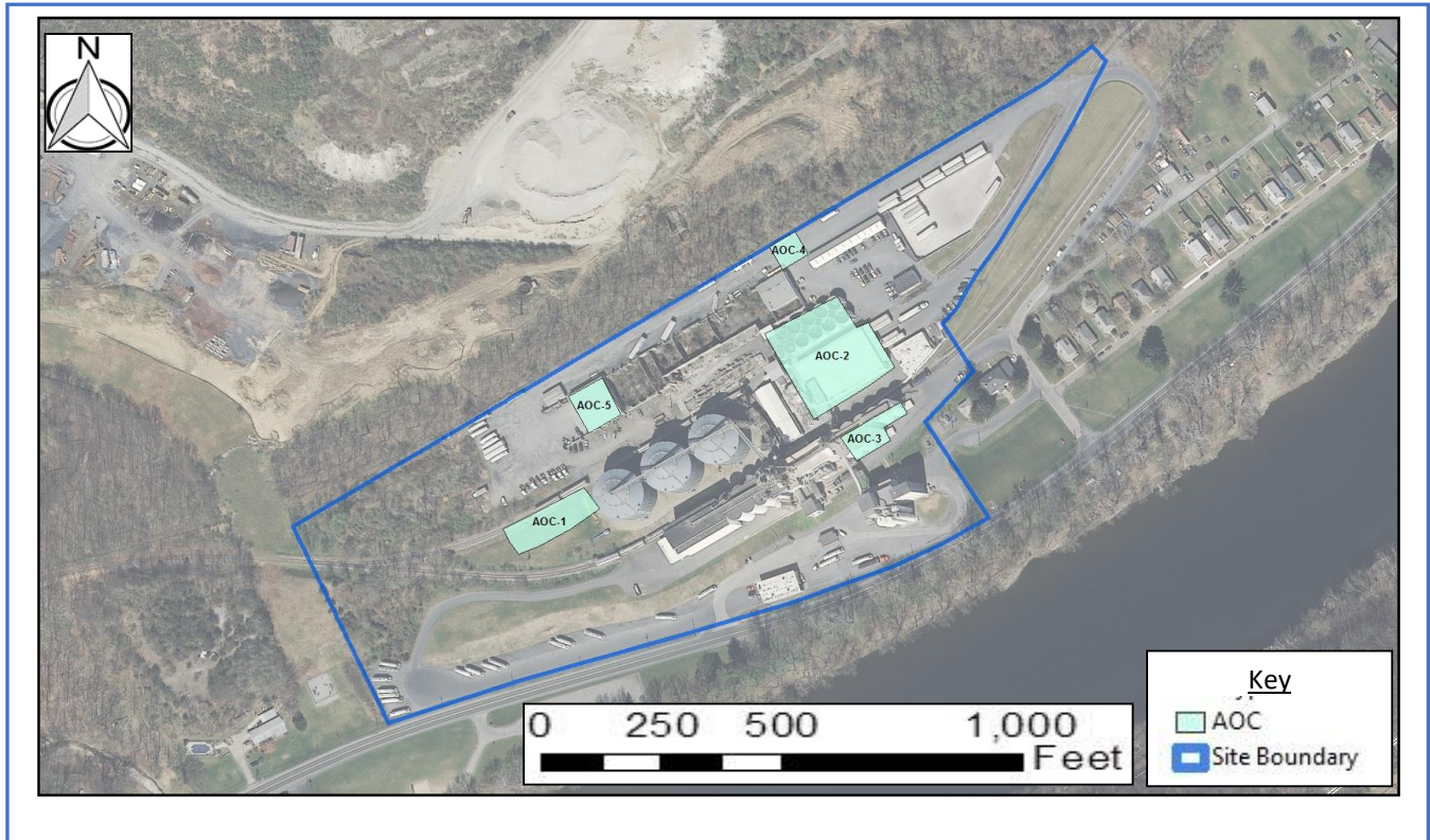
Figure 4. Map of the Shapefile used in AOC Deliverable example. The six polygons depict the Site Boundary and the 5 AOCs at the fictitious ABC Industry Site.
