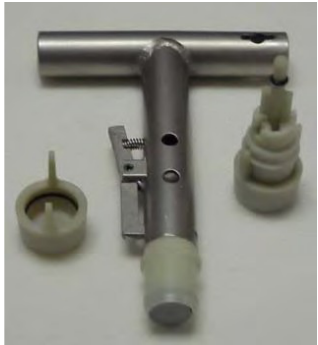
Figure 5.36 En Core® Sampler with T Handle (Photograph by C. Van Sciver)
