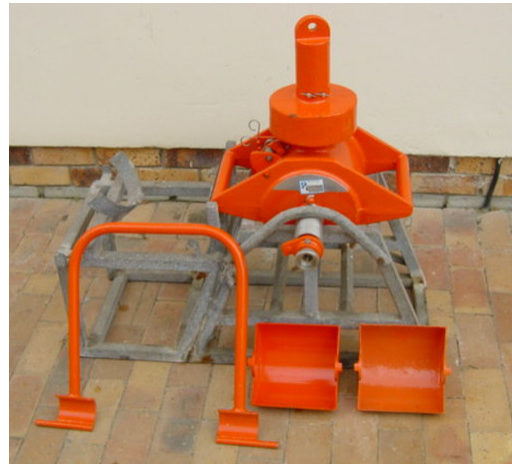
Figure 5.40 Shipek® Grab Sampler. Illustration published with permission of Wildco®
