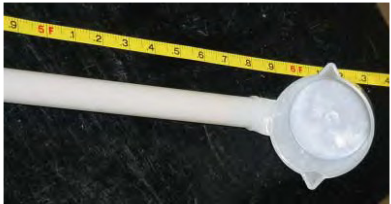
Figure 5.20 Pond Sampler (Photograph by J. Schoenleber)
