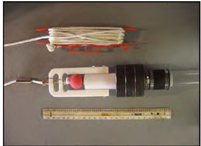
Figure 5.47 Gravity Corers. Illustration published with permission from Aquatic Research Instruments
