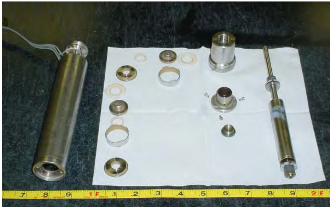
Figure 5.4 Grundfos® Pump being prepared for decontamination (Photograph by J. Schoenleber)
