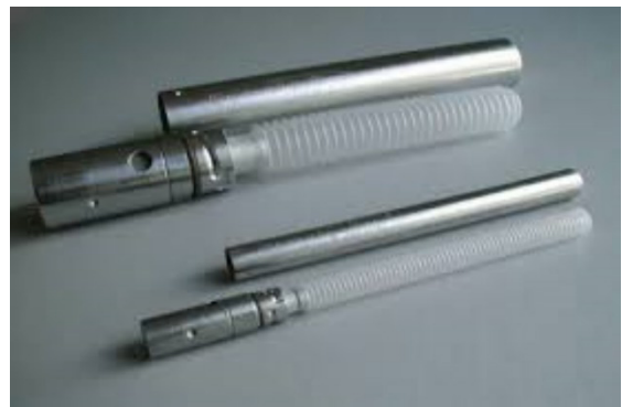
Figure 5.2 Bladder pump with a polyethylene bladder
