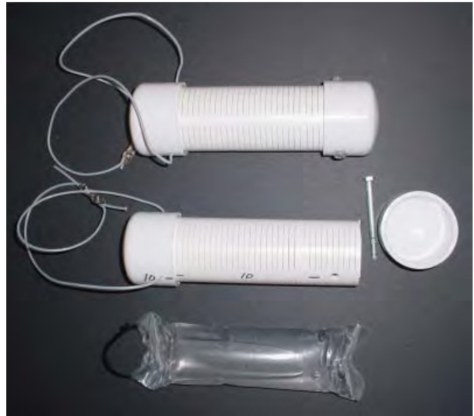
Figure 5.18 PDB for Sediments using bag provided by Columbia. (Photograph by J. Schoenleber)
