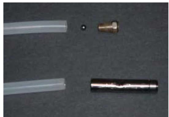
Figure 5.10 Two styles of foot check valves offered by Geoprobe® for narrow diameter temporary well points (Photograph by J. Schoenleber)
