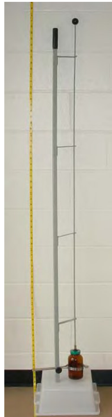
Figure 5.23 Wheaton Dip Sampler (Photograph by J. Schoenleber)
