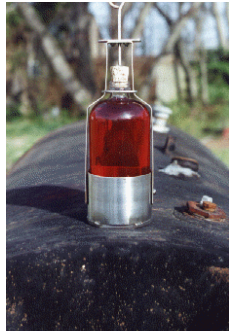
Figure 5.22 Weighted Bottle Sampler.
