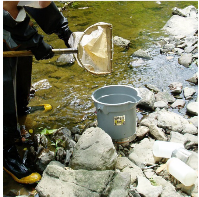
Figure 6.14. D-Frame Net. The bottom of the net is flat to facilitate getting the net close the bottom.
