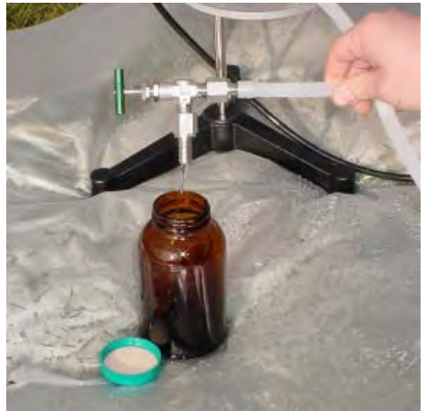
Figure 6.12 Closeup of Needle Valve. (Photograph by D. Dibblee)
