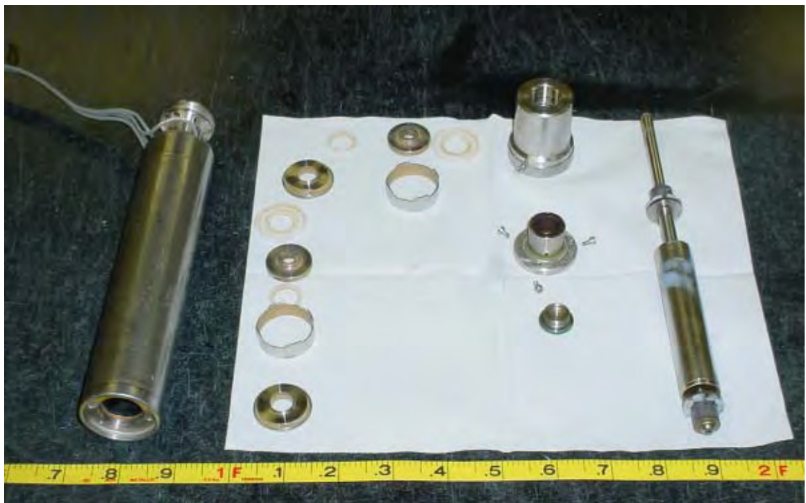
Figure 6.13 Grundfos® Pump being prepared for decontamination (Photograph by J. Schoenleber)
