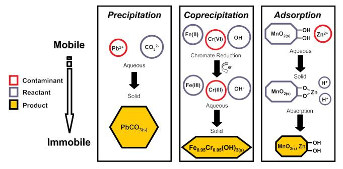
Figure 2.4 Examples of contaminant-specific sorption processes that may lead to attenuation of the ground-water plume. Color coding is employed to distinguish the contaminant (red), aqueous or solid phase reactants (blue), and the product (yellow) of the reaction leading to contaminant attenuation. Absorption is illustrated as a possible sequential process that follows the adsorption of a contaminant onto a mineral component within aquifer solids.
