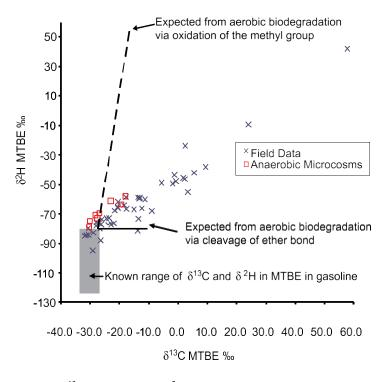
Figure 4.4. Concurrent analysis of  $\delta^{13}$ C in MTBE and  $\delta^{2}$ H in MTBE in ground water to associate natural biodegradation of MTBE in ground water with an anaerobic process, which allows the selection of an appropriate value for the enrichment factor ( $\epsilon$ ) to be used to estimate the extent of biodegradation of MTBE.
