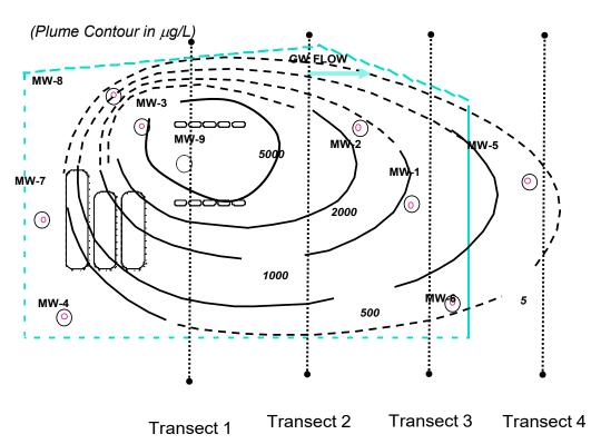
4. Estimating the mass flux of the contaminant crossing a transect ( $\dot{l}$ ) using the following equation (Eq. D.1);
