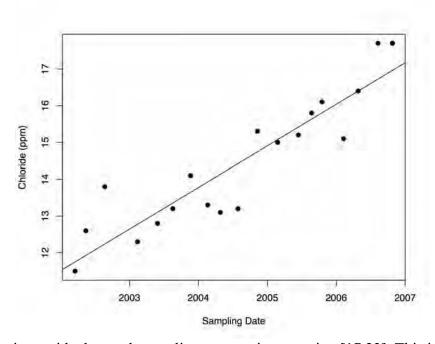
Step 2. Calculate the regression residual at each sampling event using equation [17.23]. This involves computing an estimated concentration along the regression line for each sampled time (t) and then subtracting from the observed concentration. For example, the residual at t = 407 is
