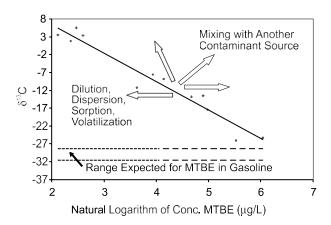
Figure 4.2. Testing field data on CSIA and concentrations of contaminants for fit to the Rayleigh equation. Deviations from a straight regression line in the plot of  $\delta^{13}$ C on the natural logarithm of concentration can indicate that processes other than degradation control the concentrations of contaminants. Example data plotted for Table 1 of Kolhatkar et al. (2002). The dotted lines bound the values of  $\delta^{13}$ C that are expected for MTBE that was blended into gasoline.
