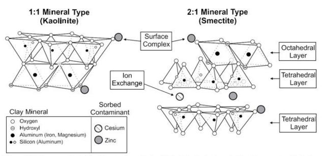
Figure 2.5 Diagrammatic sketch of the structure of 1:1 and 2:1 phyllosilicate minerals. Also shown are hypothetical sorption reactions for zinc and cesium (ion exchange represented as 'M<sub>x</sub>' in structural formulas for 2:1 phyllosilicates shown in text).
