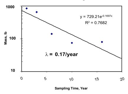
Figure D.8. Estimation of Biodegradation Rate Constant from Mass Change over Time
