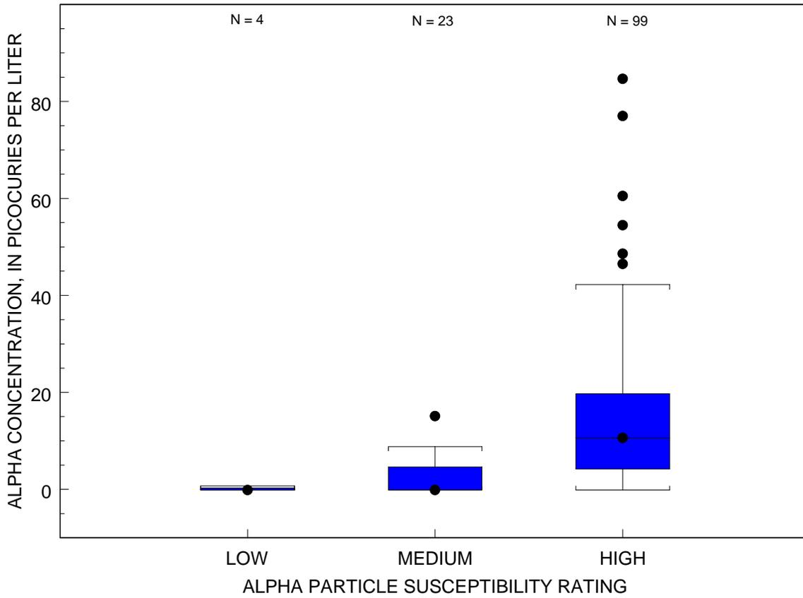
Figure 17A. Results of the gross alpha-particle activity susceptibility assessment model for 126 community water-supply wells in New Jersey showing distribution of gross alpha-particle activity by susceptibility rating.
