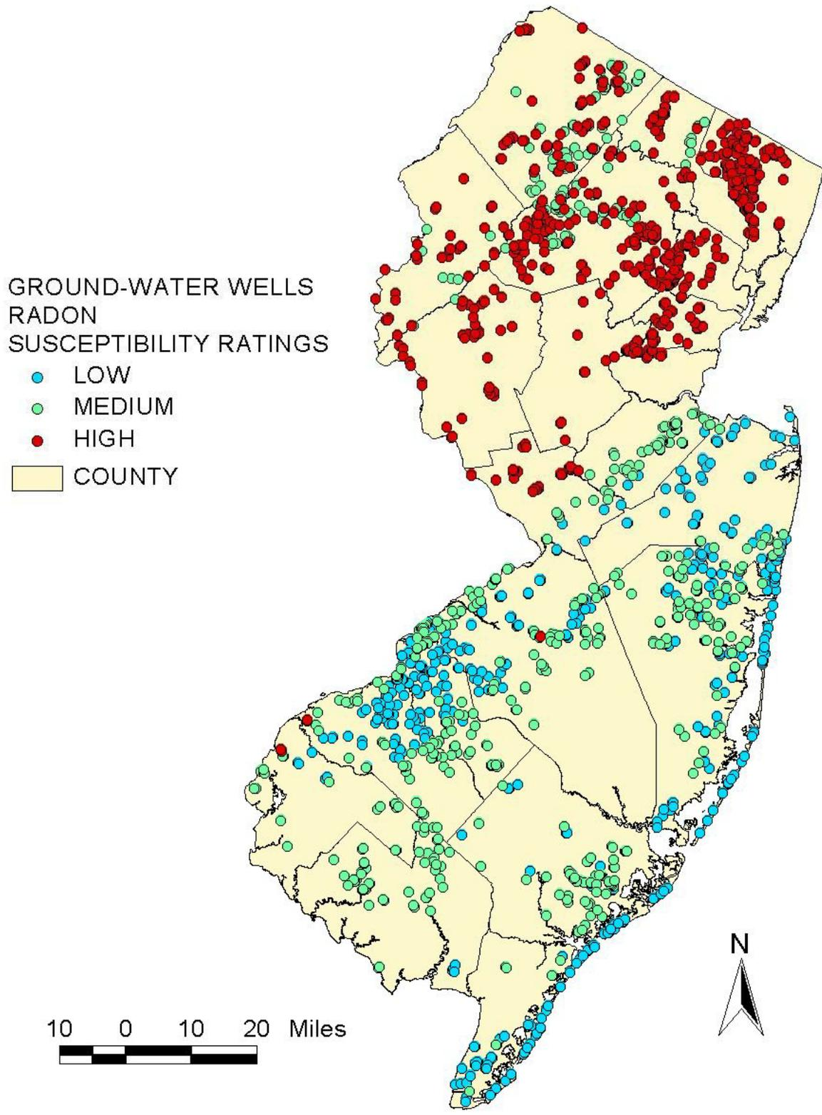
Figure 2. Susceptibility of 2,237 community water-supply wells in New Jersey to contamination by radon.
