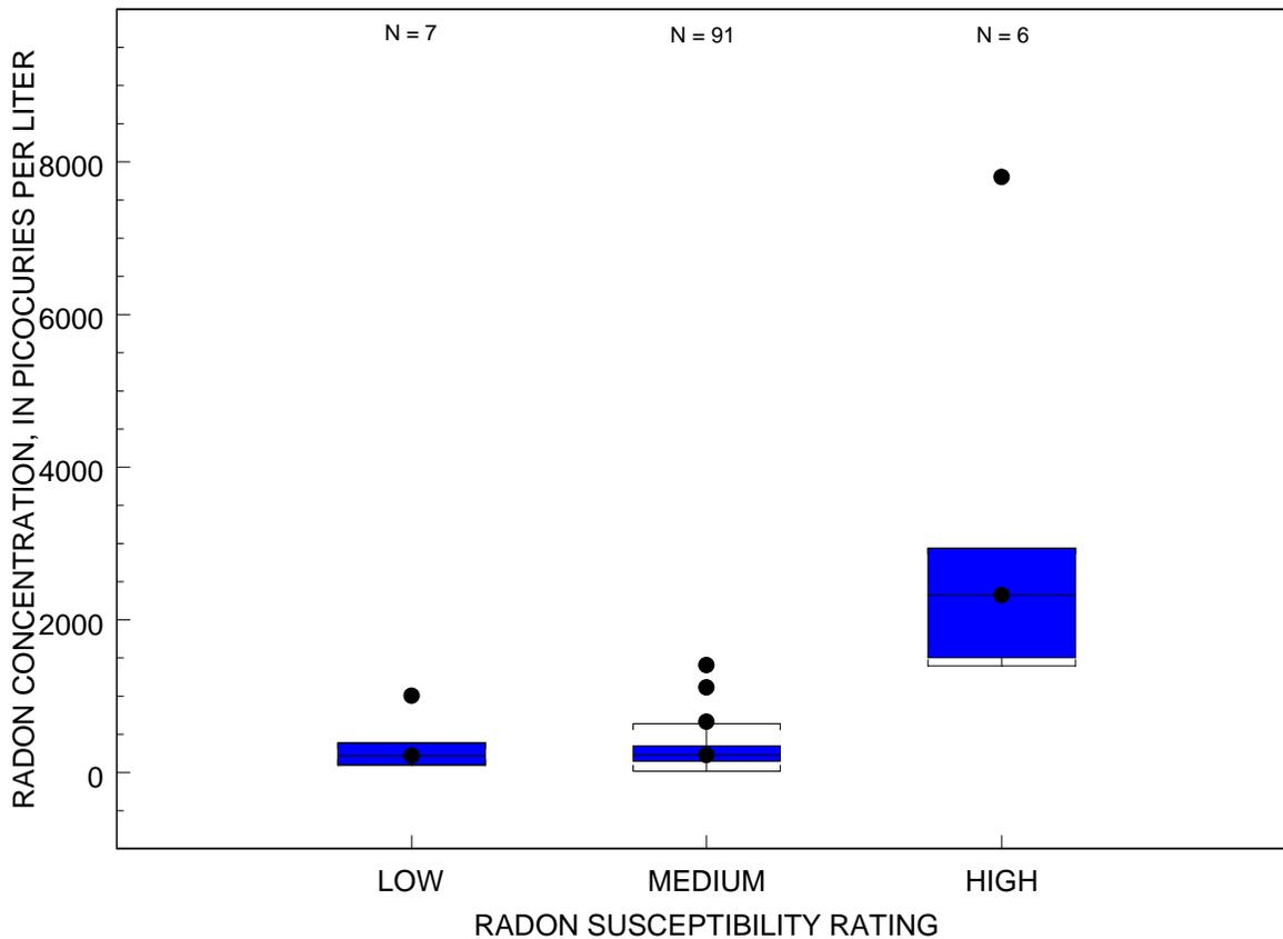
Figure 17D. Results of the radon susceptibility assessment model for 104 community water-supply wells in New Jersey showing distribution of radon concentration by susceptibility rating.
