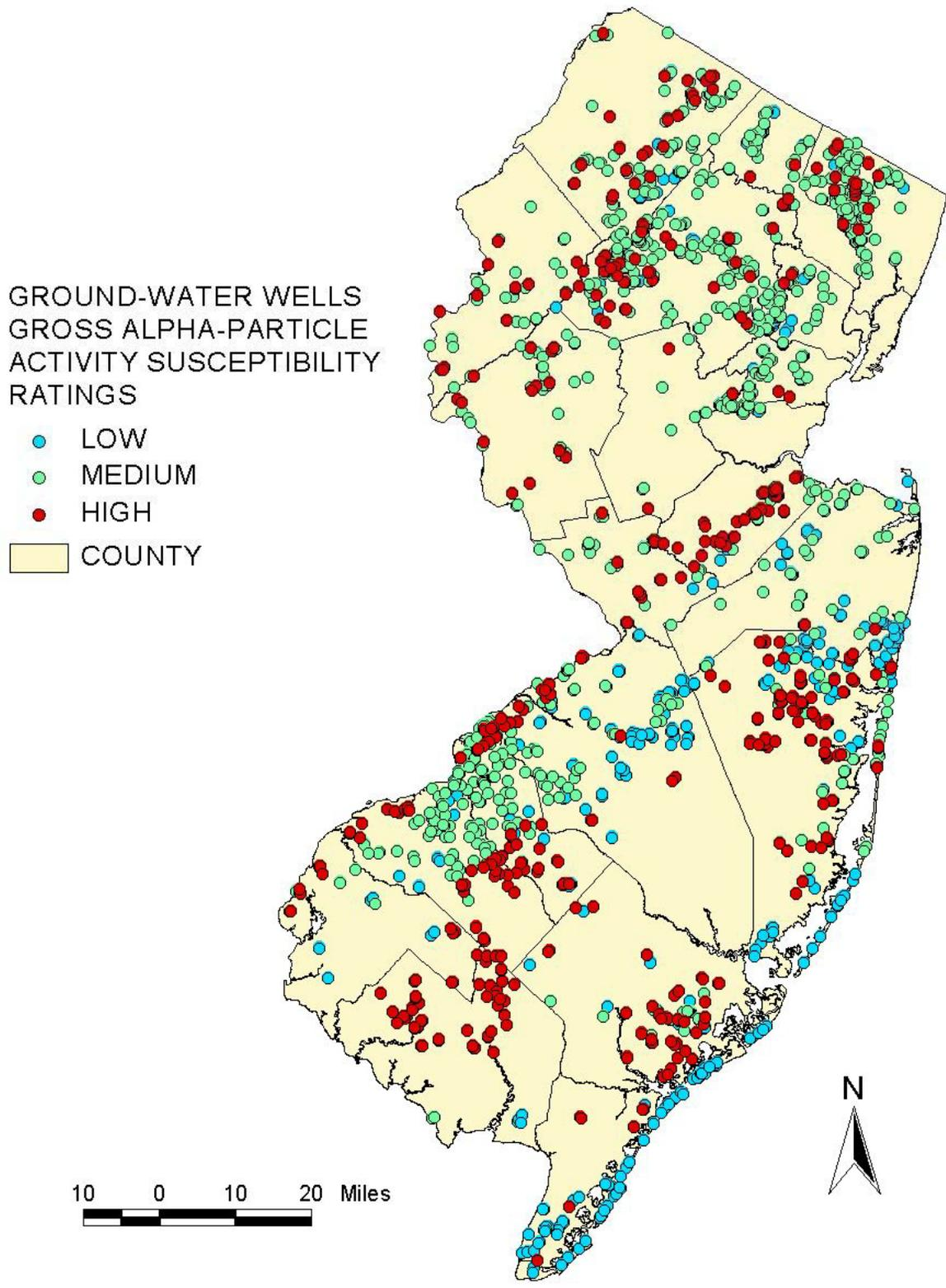
Figure 8. Susceptibility of 2,237 community water-supply wells in New Jersey to contamination by gross alpha-particle activity.
