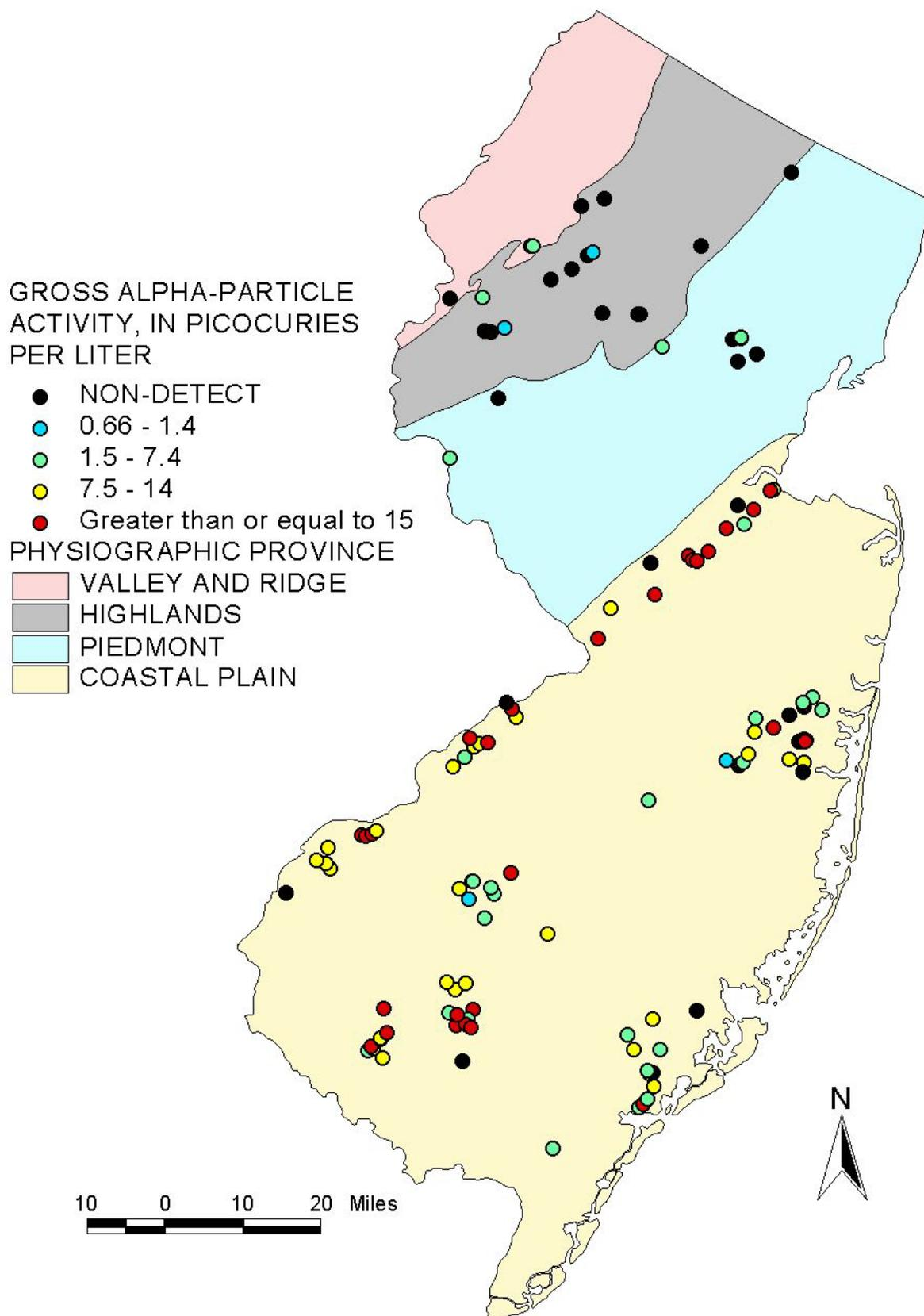
Figure 6. Gross alpha-particle activity in 126 community water-supply wells used for development of the gross alpha-particle activity model.
