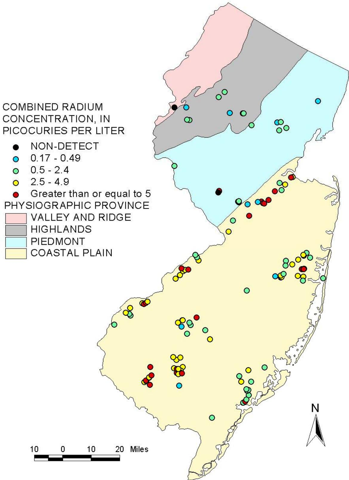
Figure 9. Concentrations of combined radium in 126 community water-supply wells used for development of the combined radium model.
