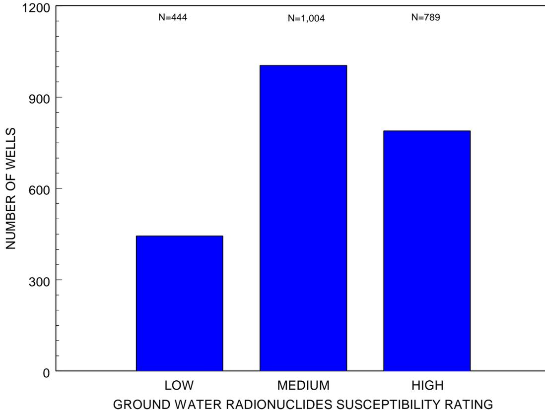
Figure 3. Number of community water-supply wells in New Jersey having low, medium, and high susceptibility to contamination by naturally occurring radionuclides (excluding radon).
