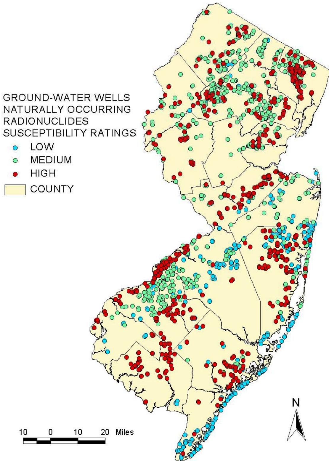
Figure 1. Susceptibility of 2,237 community water-supply wells in New Jersey to contamination by naturally occurring radionuclides (excluding radon).
