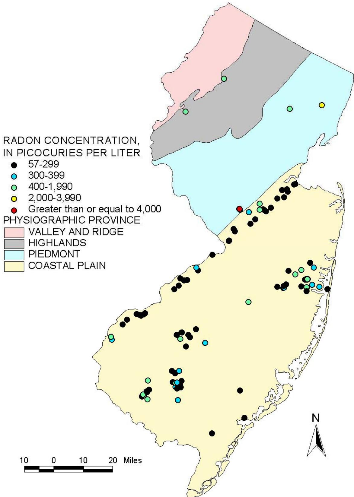
Figure 15. Concentrations of radon in 104 community water-supply wells used for development of the radon model.
