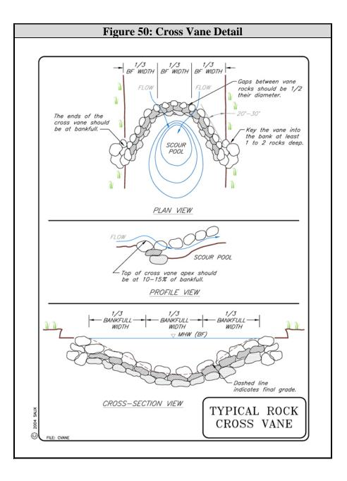
The removal of the stream obstruction located in the watershed (Figure 51) would certainly require a grade control structure post-removal, likely a cross vane. In this setting a cross vane would stabilize any head cut, connect the hydraulic jump above and below the obstruction, and align flow through the center of the channel.
