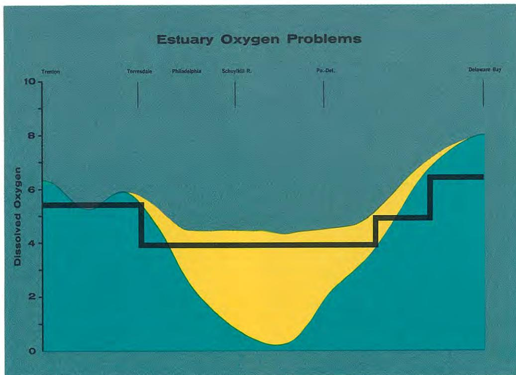
**DISSOLVED OXYGEN** is a main water purity measure. Levels below 4 (parts per million) harm fish and aquatic life, with kills occurring more often as oxygen drops. Chart shows (bottom line) typical warm weather oxygen sag in Delaware estuary; (straight line) the oxygen criteria specified in Commission's new standards; and (top line) projection of oxygen when the standards are achieved.
