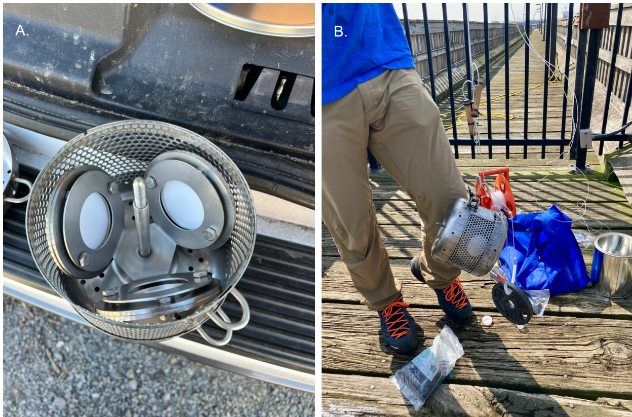
Figure 3. A) POCIS membrane triplicate resting inside of a stainless-steel canister prior to deployment. B) Closed sampler canister prior to deployment.
