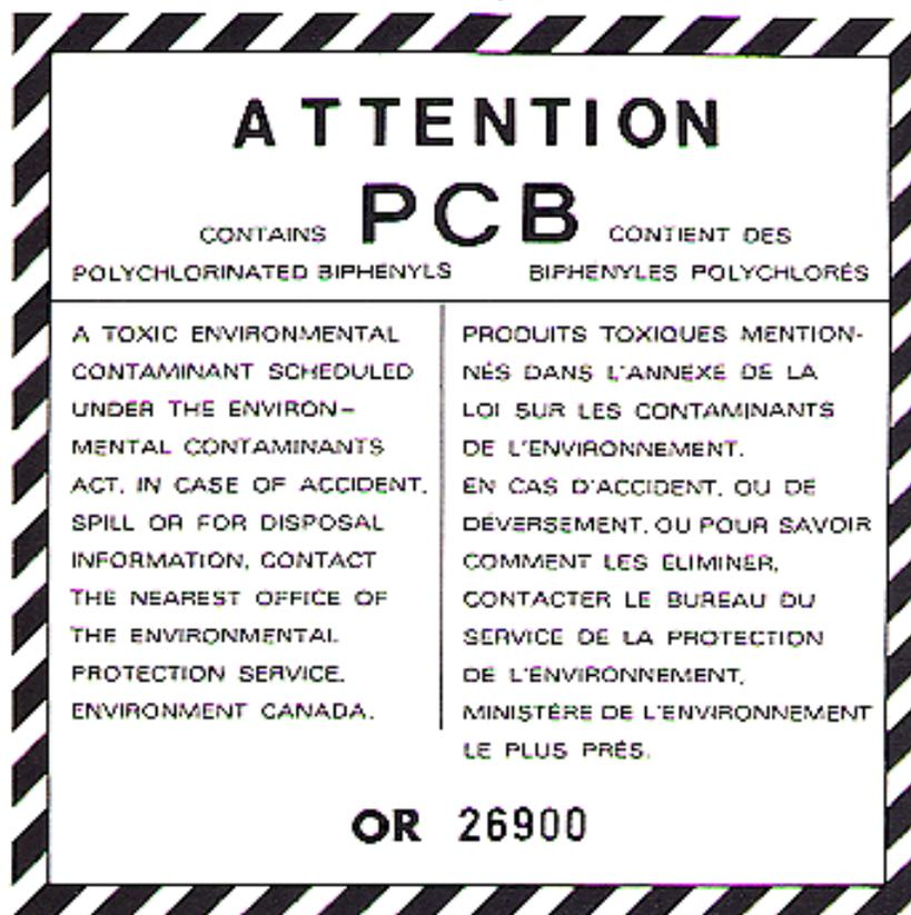
Figure 5a) Label for Large Equipment (e.g., Transformers)
