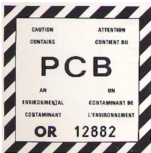
Figure 5b) Label for Small Equipment (e.g., Capacitors)
