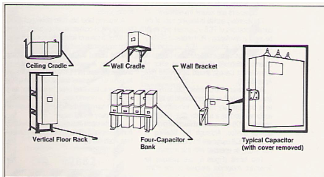
**Figure 4 Typical Indoor Capacitors**
