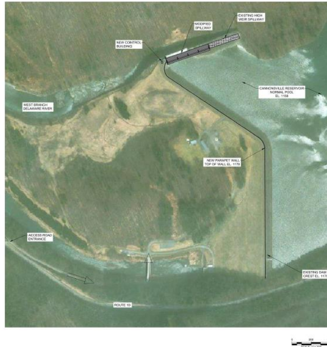
Figure 3.1: Overview of dam and spillway modifications
