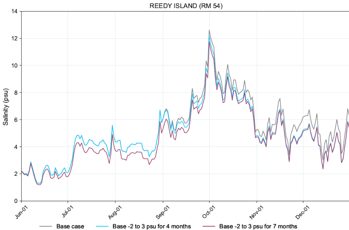
Figure C.3-4 Simulated Daily Depth-averaged Salinity at Reedy Island (RM 54) during June through December 2017: Sensitivity to Salinity at Ocean Boundary
