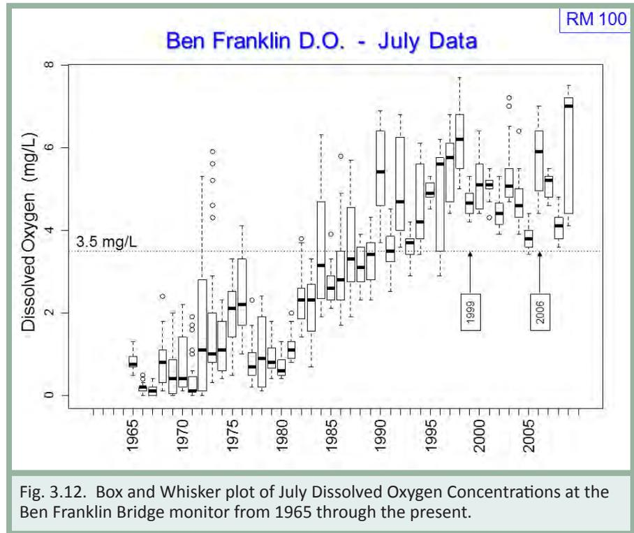
Fig. 3.12. Box and Whisker plot of July Dissolved Oxygen Concentrations at the Ben Franklin Bridge monitor from 1965 through the present.
