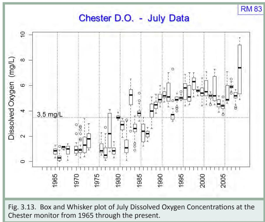
Fig. 3.13. Box and Whisker plot of July Dissolved Oxygen Concentrations at the Chester monitor from 1965 through the present.
