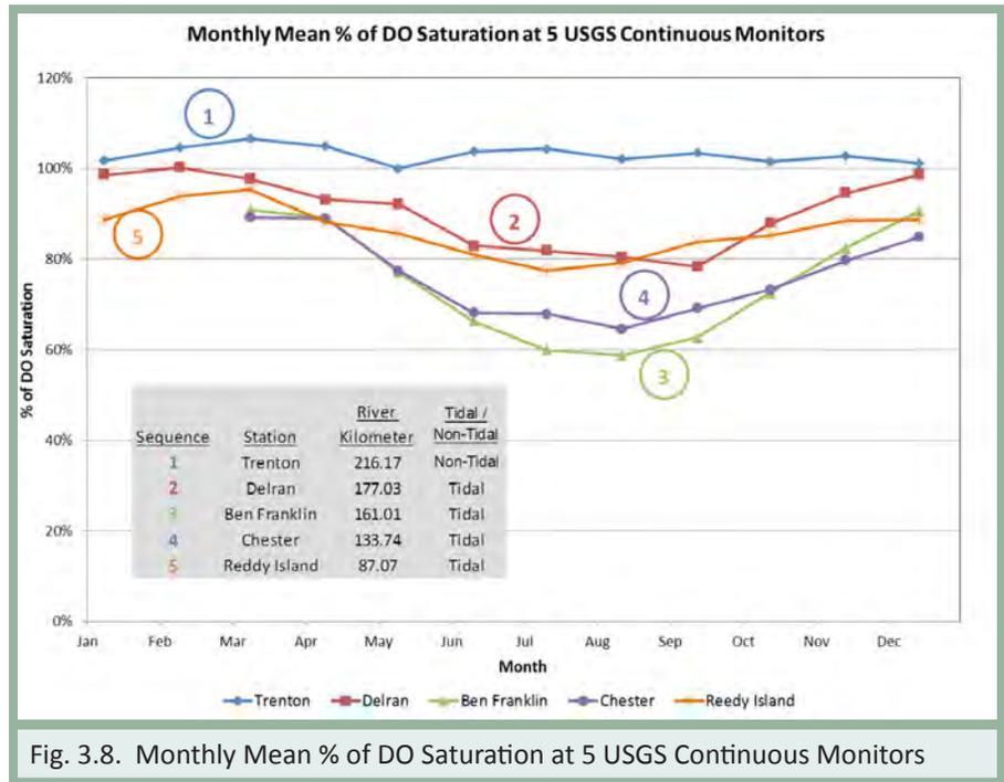
Fig. 3.8. Monthly Mean % of DO Saturation at 5 USGS Continuous Monitors
