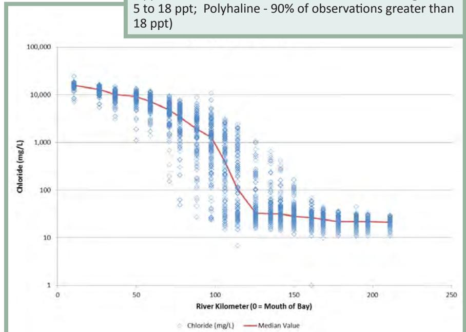
Fig. 3.33. Chloride Concentration Ranges by River Kilometer.
