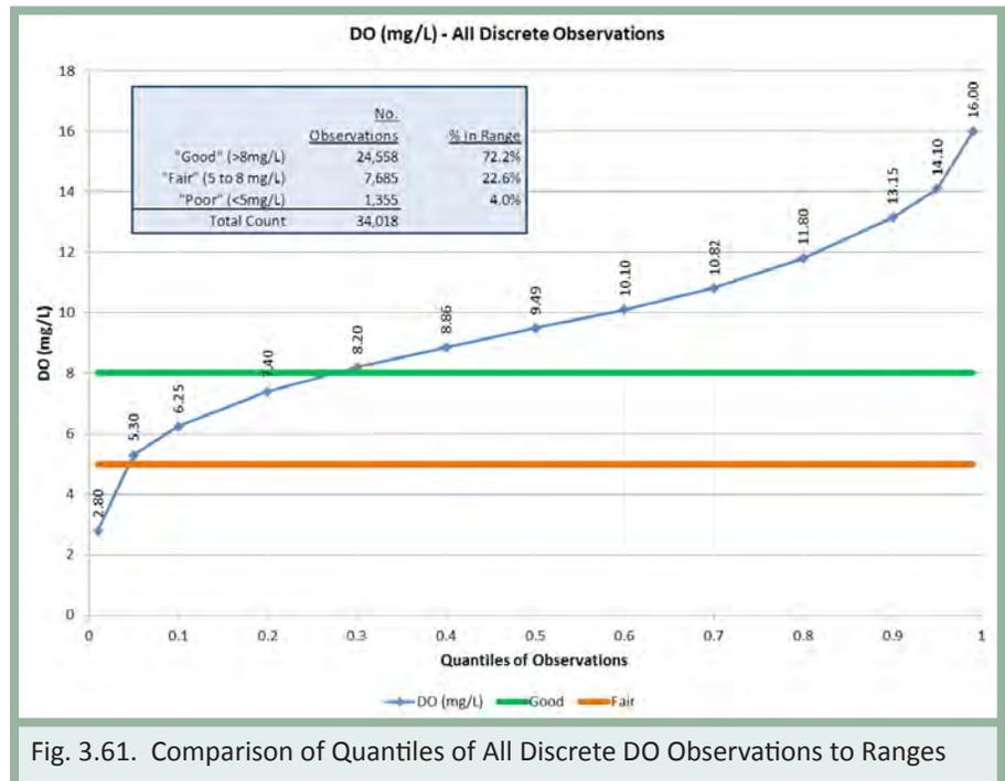
Fig. 3.61. Comparison of Quantiles of All Discrete DO Observations to Ranges
