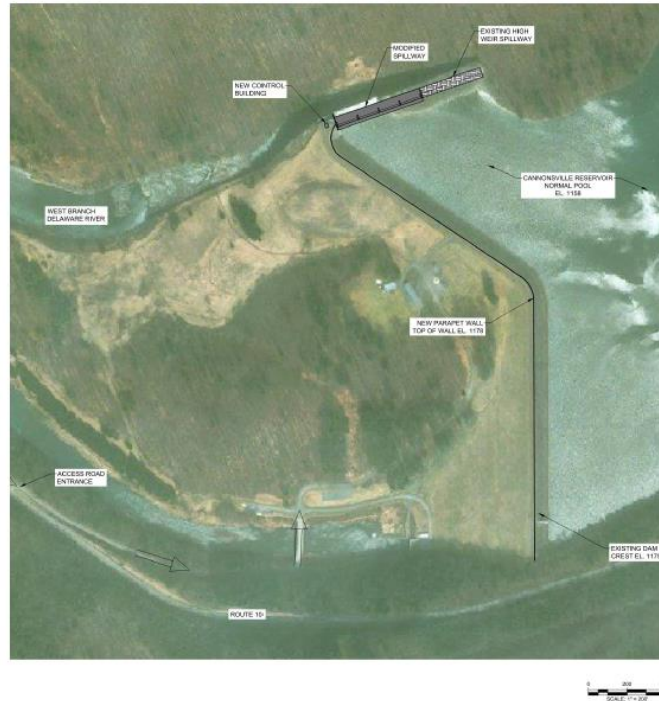
Figure 3.1: Overview of dam and spillway modifications
