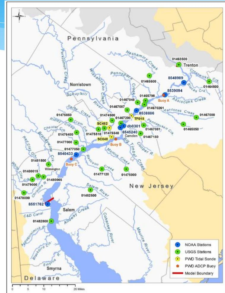
Figure 2-4: Water Level and Current Observation Meters in the Model Domain
