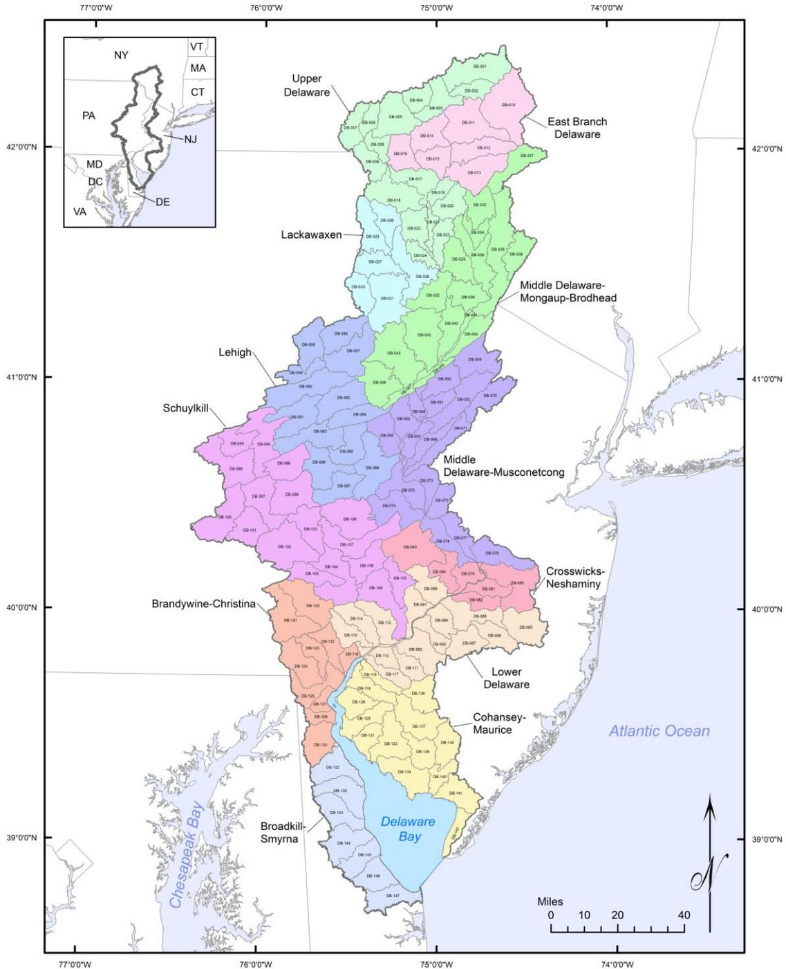
**Figure 5:** A map of the twelve USGS HUC-8 watersheds within the Delaware River Basin, and the 147 modified sub-watersheds representing drainage areas ranging in size from 17.9 to 210 mi<sup>2</sup>, as were defined in *Sloto & Buxton, 2006*.
