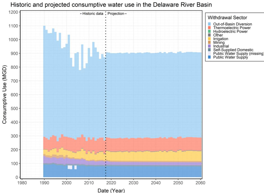
**Figure ES-2: Historical and projected consumptive water use in the Delaware River Basin.** Data in this figure has been provided in data releases corresponding with each sector. The historical data and projection have been color coded by sector to demonstrate the relative magnitude and trends of the expected value.
