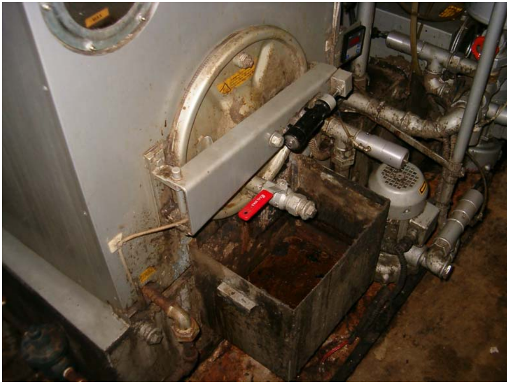
Photograph 5: Back of Realstar dry cleaning machine showing cleanout chamber.
