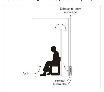
contained airflow and recirculation system (see Environmental Controls; Figure 2).
