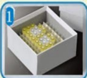
Place the absorbent material in the bottom of the gridded box and carefully insert the cryotubes
