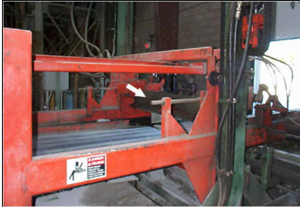
Cubing machine showing stationary bolt
