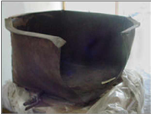
Photo 2 Acid Tank Involved in Incident
