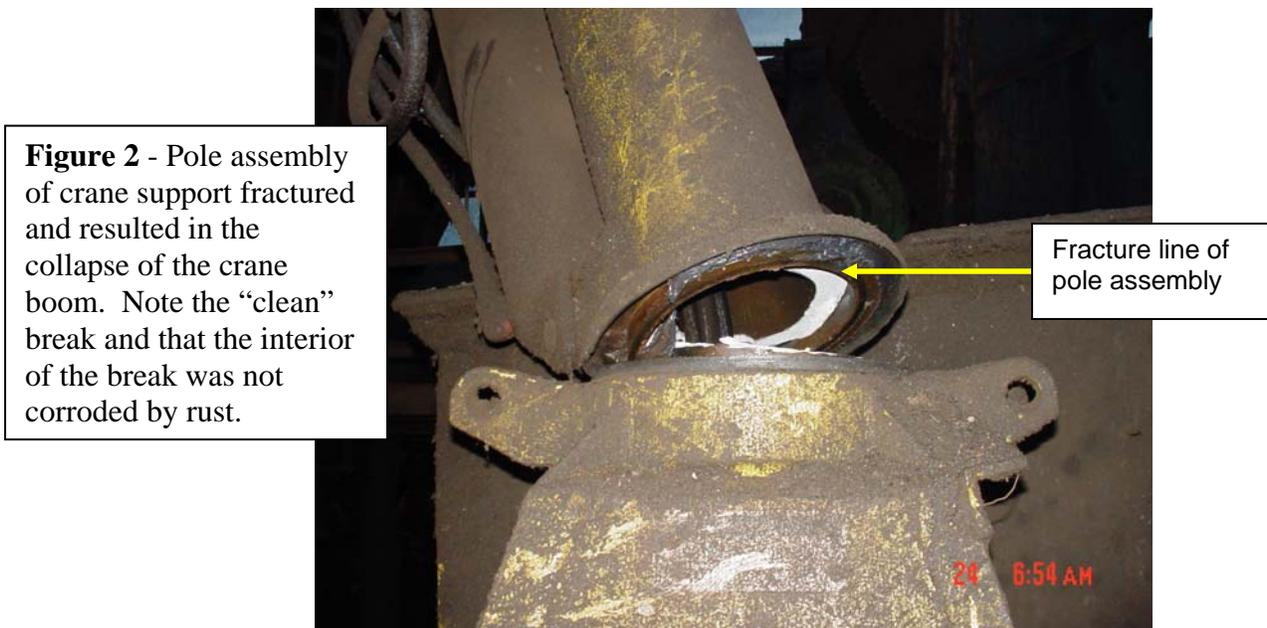
A lack of understanding and control of the crane's load limits was probably a significant contributing factor to the crane failure. The procedure followed to remove jams from the hammer mill did not allow for a means to determine the force and load exerted on the crane, potentially giving rise to situations where the rated maximum load capacity of the crane was exceeded. Over time, the structural integrity of the crane deteriorated, resulting in its eventual failure.
