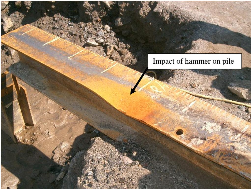
Figure 4: Pile as it rested after crushing victim. Note the muddy conditions.
