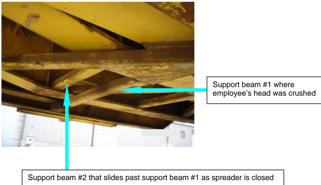
The guide rails of the telescoping sections slide through guide blocks in the middle section and allow the sections of the spreader to maintain alignment when being opened and closed. In addition, the telescoping sections of the spreader have structural support beams on the underside of the spreader (see Figure 4).
