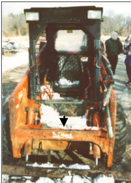
**Arrow points to cross member of boom lift-arm assembly of the skid-steer loader.**
