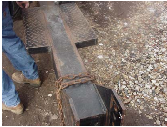
Improperly Modified Yoke
