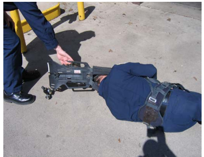
Crack At Lumbar Support Caused Separation Failure
