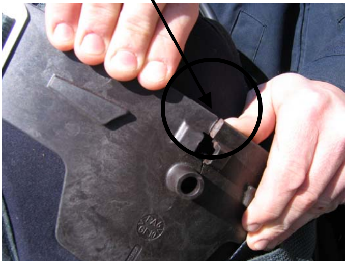
Crack From Pulling & Dragging
