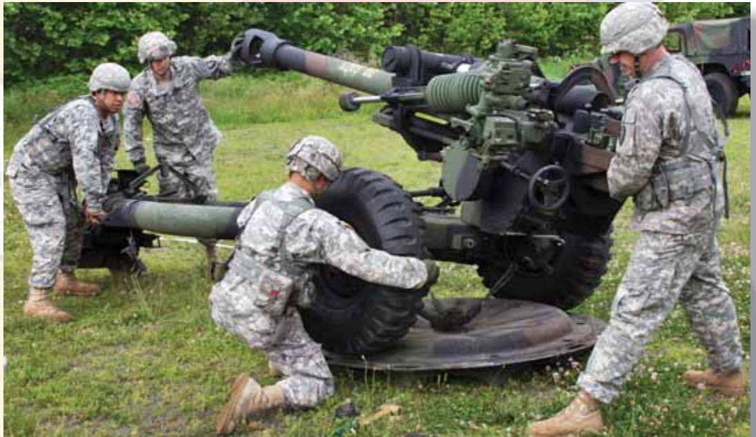
Soldiers from 1st Platoon, Alpha Battery, 3-112th Fires Battalion place an M119 105mm Howitzer during a platoon occupation exercise June 8, 2012 at the Morristown, N.J. armory in preparation for Annual Training.
