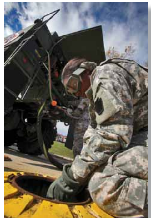
Pvt. Andrea Pittman, 1-150th Assault Helicopter Battalion, offloads 1,000 gallons of diesel fuel from a Heavy Expanded Mobility Tactical Truck M978 2,500 gallon fuel tanker at the municipal fuel depot at Morris Township, N.J. Nov. 3, 2012. (Air National Guard photo by Master Sgt. Mark C. Olsen/Released)
