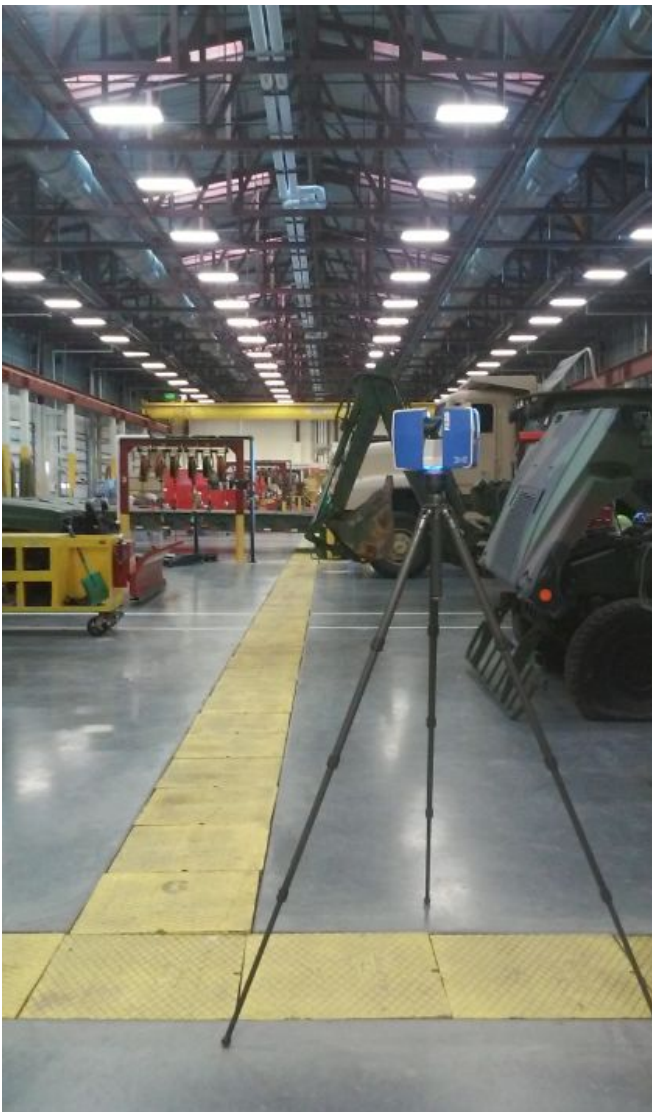
Left: Faro Focus 3D X330 set up at the Lakehurst CLTF.
